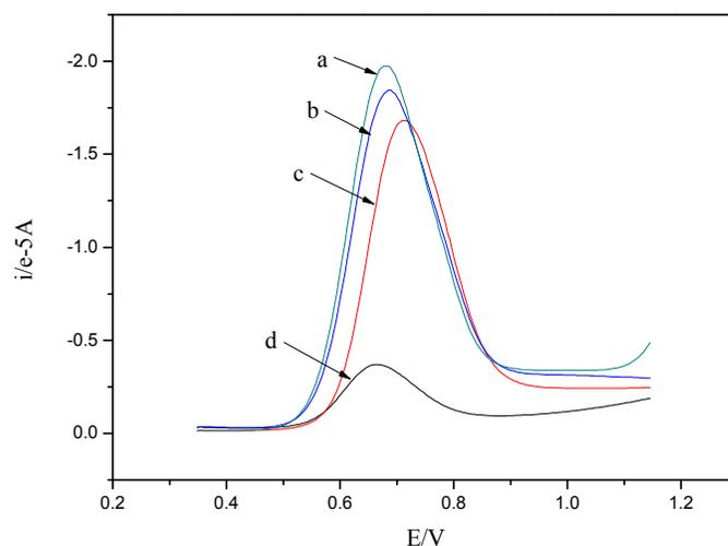
**Fig. 5** Potential voltammograms of the D- or L- Trp enantiomers on the electrodes: (a) D-Trp on GCE; (b) L-Trp on GCE; (c) L-Trp on MWCNT-CS/GCE; (d) D-Trp on MWCNT-CS/GCE.
