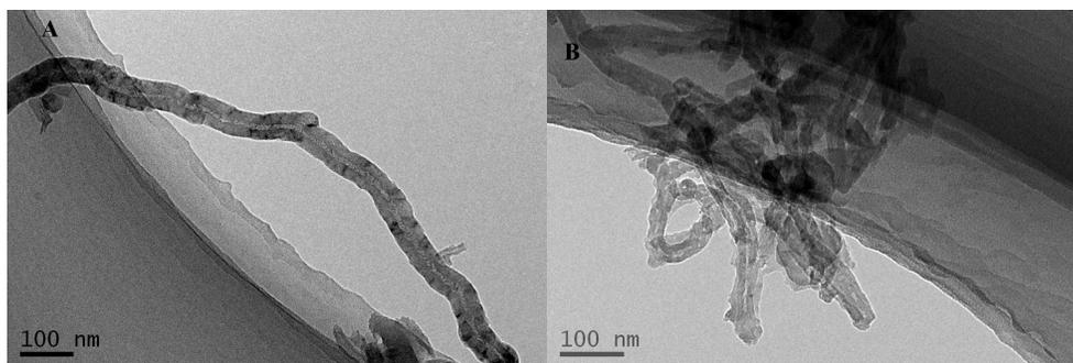
**Fig. 3** TEM images of MWCNT samples: (A) pristine MWCNTs; (B) MWCT-CS.
