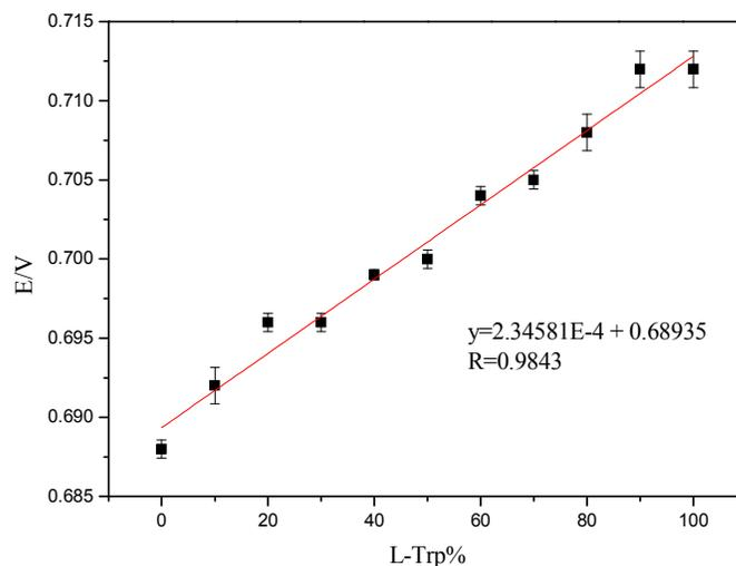
**Fig. 7.** The relationship between  $E_p$  and different percentage of L-Trp (%) of 2.5 mM Trp racemic mixture on MWCNT-CS/GCE.
