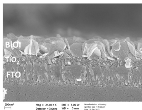
Figure 2. Cross-sectional FESEM image of a BiOI/TiO 2 /FTO photoanode, made by 15 SILAR cycles. The scale bar is 200 nm.
