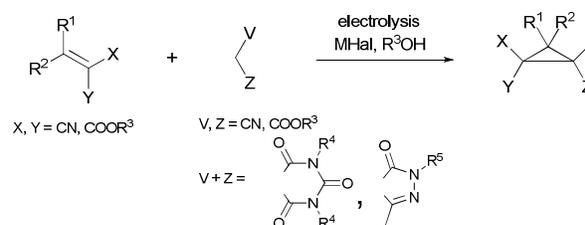
Scheme 1 Electrolysis of activated olefins and C-H acids
