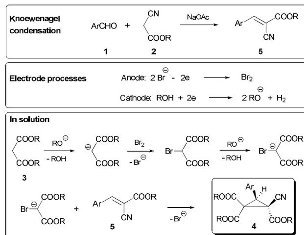
**Scheme 5** Mechanism of the electrocatalytic stereoselective multicomponent synthesis of cyclopropanes **4**.
