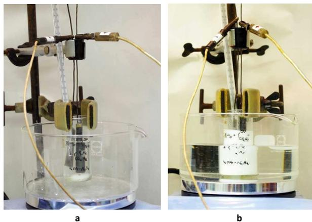
**Fig. 2** a) Start point of domino process, b) reaction mixture after premixing (the white precipitate is methyl benzylidenecyanoacetate **5**).
