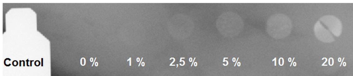
Figure 4. Ex vivo X-ray images of PCL-TIB/PLA 50 - b -PEG- b -PLA 50 blends implanted in a 4 cm thick anatomical model. Control corresponds to 2 mm thick aluminum wedge. Percentages correspond to iodine weight ratios (20 wt% sample film shown is broken in two pieces; dark line in the middle of the sample corresponds to this fracture).
