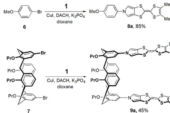
Scheme 2 Copper catalyzed *N*-arylation reaction using MPTTF **1**. DACH = *trans*-1,2-diaminocyclohexane.
