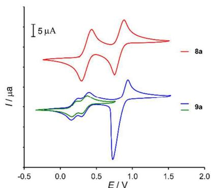
Fig. 3 Cyclic voltammograms of compounds **8a** (red) and **9a** (blue). For **9a**, the green curve shows a CV scan centered on only the first two oxidation potentials of the TTF moieties. (Plotted vs. SCE;  $\text{CH}_2\text{Cl}_2/0.1 \text{ M Bu}_4\text{NClO}_4$ ).
