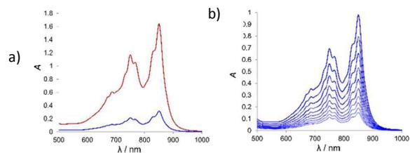
Fig. 5 a) Comparison between the charge-transfer bands of molecular complexes of receptors **9a** (red) and **9b** (blue) with TCNQ ( $\text{CH}_2\text{Cl}_2$ ,  $[\mathbf{9}] = [\text{TCNQ}] = 2 \times 10^{-4} \text{ M}$ ); b) UV/Vis spectra of dilution of 1:1 receptor **9a** / TCNQ mixture ( $\text{CH}_2\text{Cl}_2$ ,  $[\mathbf{9a}] = [\text{TCNQ}] = 1.25 \times 10^{-4} - 2.42 \times 10^{-5} \text{ M}$ ).
