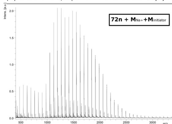
**Figure 2.** MALDI-ToF MS spectrum of PDLA oligomers synthesized with non-dried N345 as catalyst.
