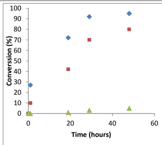
**Figure 3.** Monomer conversion ▲ L-lactide without enzymes, ◆ with N435 –on D-lactide and ■ with LBC on L-lactide
