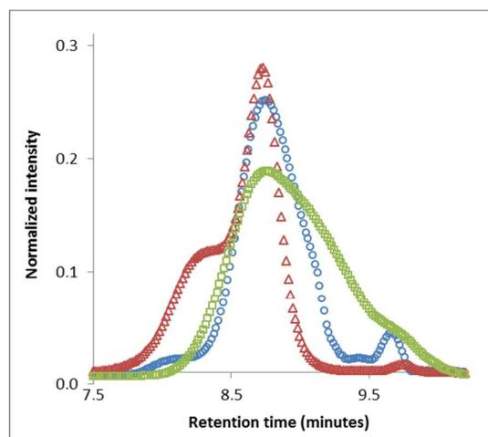
Figure 7. SEC elution profiles of PLA produced by eROP catalyzed by N435 in toluene:triethylamine solvent mixture. After 8h (○), 24h (△) and 48h (□) of reaction. All curves were normalized on flow marker intensity.
