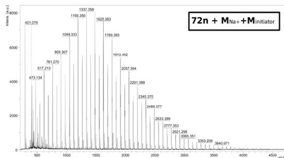
Figure 5. MALDI-ToF spectrum of PDLA oligomer synthesized with dry N435
