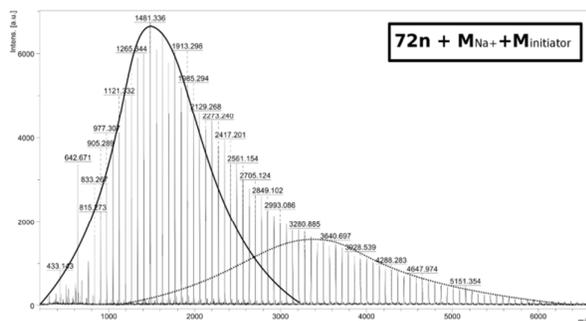
**Figure 8.** MALDI-ToF spectrum of PDLA oligomer synthesized with dry N435 in toluene:TEA mix
