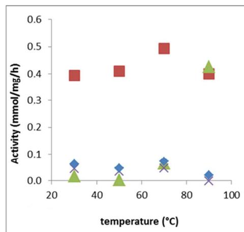
Figure 1. Enzymatic activity for oleic acid esterification by octanol (expressed in mmol of ester formed per mg of enzyme and per hour) at various temperatures; ■ N435; ▲ LBC; × LCR; ◆ PPL.
