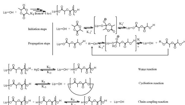
**Charts 1.** Mechanism and reaction pathways for enzymatic ring opening polymerization of lactide, adapted from PM Johnson and coworkers [38]
