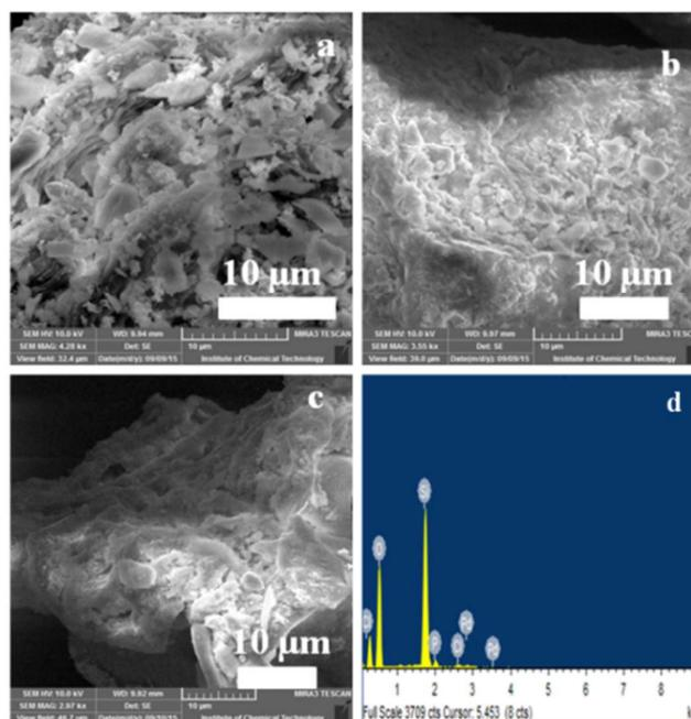
**Fig. 2** FEG-SEM images of (a) Fresh, (b) 1<sup>st</sup> recycled (c) 4<sup>th</sup> recycled PdCl<sub>2</sub>/PPh<sub>2</sub>Et@SiO<sub>2</sub> catalyst and (d) EDS spectrum of Fresh catalyst.
