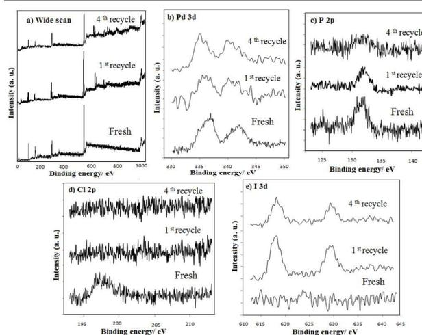
Fig. 4 (a) XPS survey spectrum; (b) Pd 3d; (c) P 2p; (d) Cl 2p and (e) I 3d for PdCl<sub>2</sub>-PPh<sub>2</sub>Et@SiO<sub>2</sub> catalyst.
