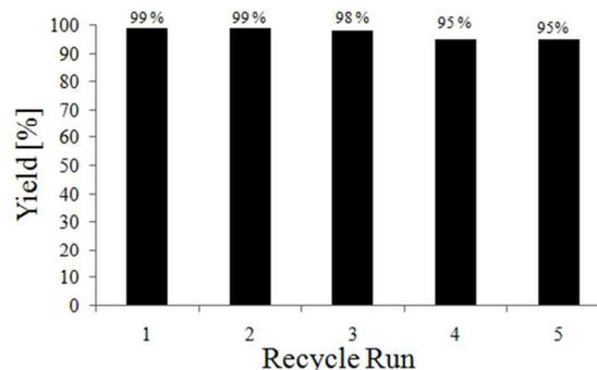
Fig. 3 Recycle study of PdCl<sub>2</sub>-PPh<sub>2</sub>Et@SiO<sub>2</sub> for alkoxy carbonylation of aryl iodide.
