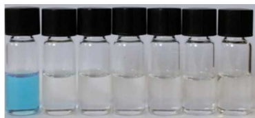
Fig. 5 Chromogenic response of SQ ( 15.0 \mu\text{M} ) with SM ( 59 \mu\text{M} with 1 conc. at 42 \mu\text{M} ) and other intereferent ( 59 \mu\text{M} ) (from left to right) sarin, soman, cyclosarin, Tabun, Vx, and BCEE.
