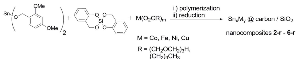
Scheme 3. STP of Si-spiro with tin(II)-2,4-dimethoxyphenylmethanolate ( 1 ) in the presence of metal containing additives gave after reduction ( \text{Ar}/\text{H}_2 , 95/5 %) the nanocomposites 2-r – 6-r .
