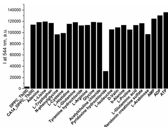
**Fig. 4** Emission intensity of DPPC-CA14-Tb(III) vesicles at 544 nm after addition of organic analyte molecules. C [CA14] = 0,07 mM; C[DPPC] = 0,7 mM; C[Tb] = 0,07 mM; C[TRIS] = 20mM; C[NaCl] = 150 mM; pH = 7,4, C[org. guest] = 0.35 mM.
