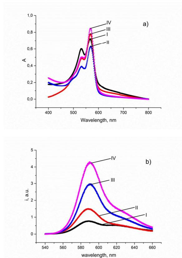
**Fig. 2** UV-VIS (a) and emission (b) spectra for vesicles: MC540-DPPC (I), MC540-CA4-DPPC (II), MC540-CA8-DPPC (III), MC540-CA14-DPPC (IV). Experimental conditions: C(CALIX) = 0,07 mM; C(DPPC) = 0,7 mM; C(MC-540) = 0,007 mM; C(TRIS) = 20mM; C(NaCl) = 150 mM; pH = 7.4, t=25°C.
