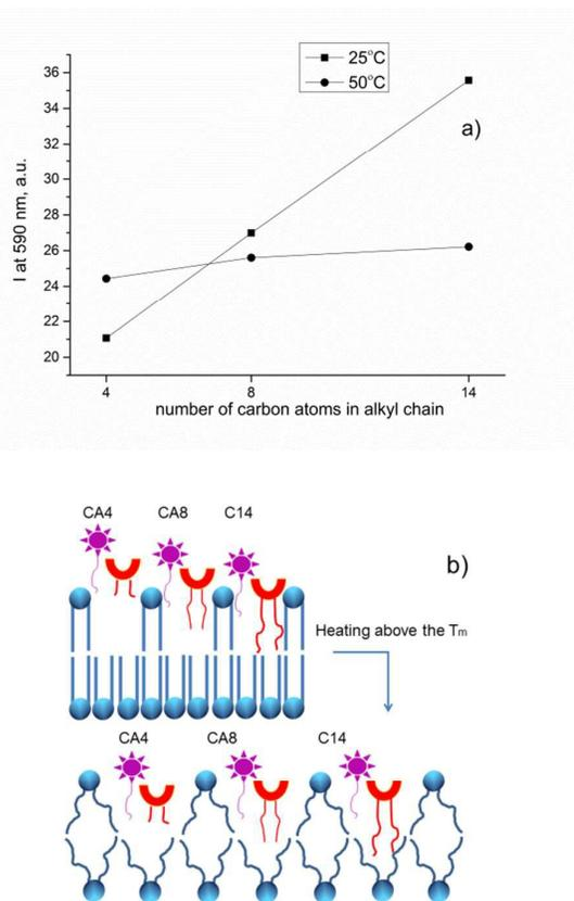
**Fig. 3** (a) Emission intensity (a.u.) at 590 nm of MC-540 embedded in CA14-DPPC vesicles at 25 and 50°C vs number of carbon atoms in calixarene alkyl chains; (b) schematic representation of calixarene-MC540 associates distribution in the bilayer below and above the normal transition temperature of pure DPPC  $T_m$ .
