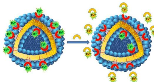
**Scheme 1.** Schematic representation of “stripping” principle of analyte detection based on calixarene-Tb(III) decorated vesicles.
