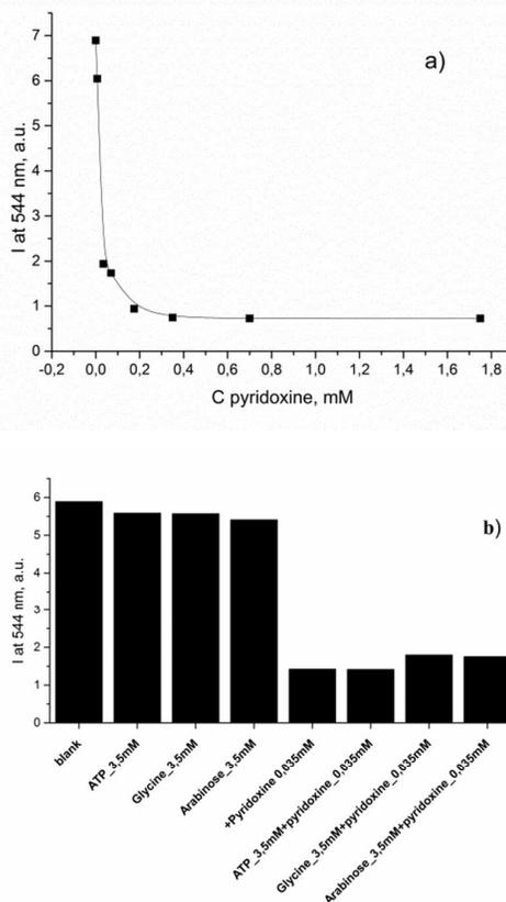
**Fig. 5** (a) Emission intensity of DPPC-CA14-Tb(III) vesicles at 544 nm vs pyridoxine HCl concentration. C[CA14] = 0,07 mM; C[DPPC] = 0,7 mM; C[Tb] = 0,7 mM; C[TRIS] = 20mM; C[NaCl] = 150 mM; pH = 7,4, C[pyridoxine] = 0,007-7 mM. (b) Emission intensity of DPPC-CA14-Tb(III) vesicles at 544 nm before/after addition of different guest mixtures, C[CA14] = 0,07 mM; C[DPPC] = 0,7 mM; C[Tb] = 0,7 mM; C[TRIS] = 20mM; C[NaCl] = 150 mM; pH = 7,4.
