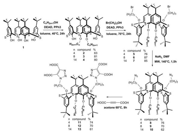
**Scheme 3.** General synthetic procedure for the synthesis of calixarene tetra-acids **11-13**
