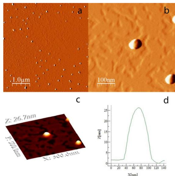
**Fig. 1** AFM topview with 5  $\mu$ m scan range (a), 0.5 $\mu$ m scan range (b); three-dimensional view (c) and size profile (d) of CA14\_DPPC vesicles with 10% mol calixarene load.
