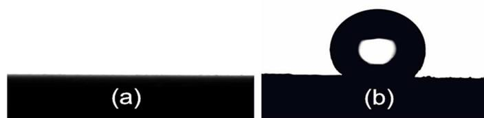
**Fig. 9** Images of surface hydrophobic behaviour of the pristine filter and the composite filter. **(a)** The water contact angle on the pristine filter. **(b)** The water contact angle on the composite filter.
