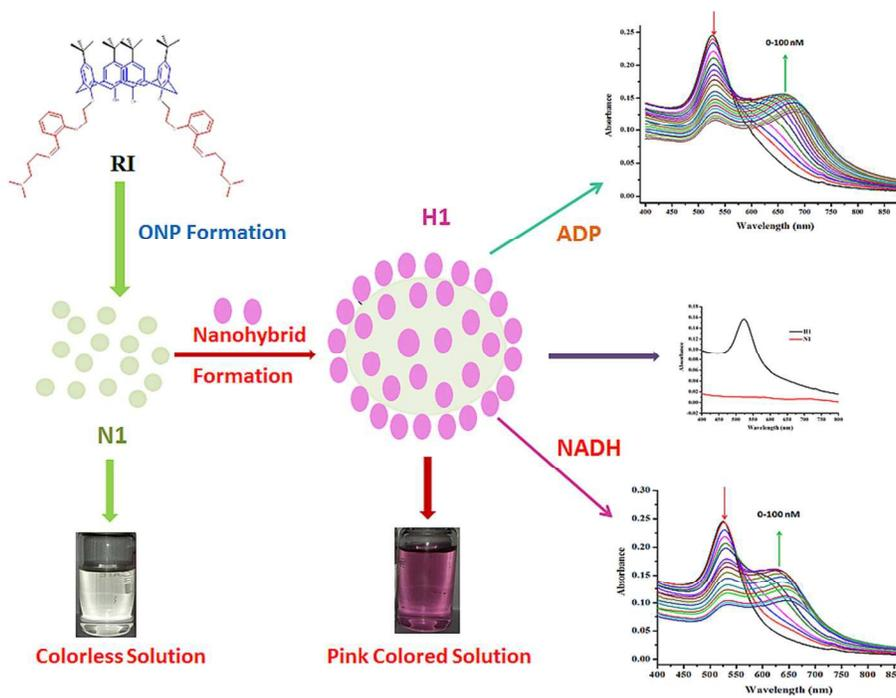
Nanohybrids of calix[4]arene based receptor has been employed for selective and simultaneous estimation of ADP and NADH.
