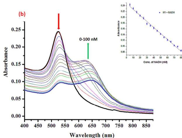
Figure 8: UV-visible Spectra of **H1** in the presence of increasing concentrations (a) (0-100 nM) of ADP, and (b) (0-80 nM) of NADH (Inset A: Calibration plot for ADP, Inset B: calibration plot for NADH)
