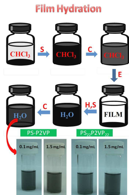
Figure 3. Film hydration exfoliation procedure of graphite in water of pH 2. (S: sonication, C: centrifugation, E: evaporation, H: hydration) and photographs of G/P hybrid stable dispersions after the last centrifugation step.
