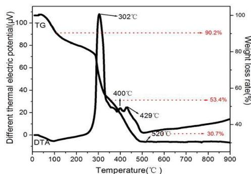
Fig. 1: Thermogravimetry-differential thermal analysis (TG-DSC) diagram for the PVP/ $\text{TiO}_2$  fibers
