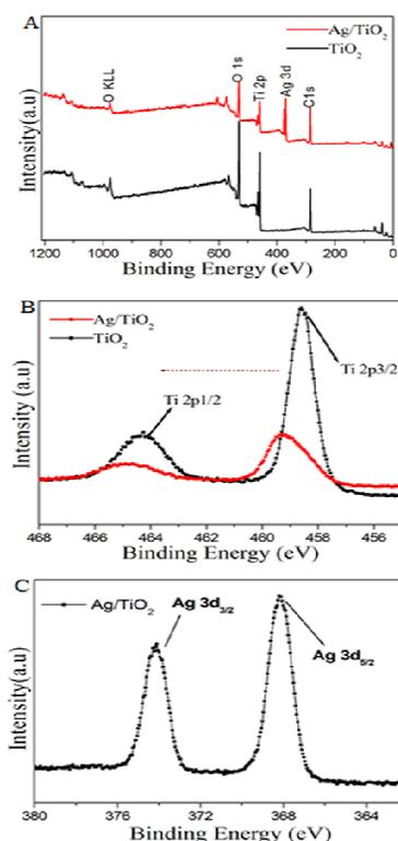
Fig. 5: The XPS spectra of Ag/ $\text{TiO}_2$  and pure  $\text{TiO}_2$  fiber (A Survey, B Ti 2p, C Ag 3d).
