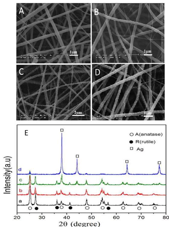
Fig. 2: The SEM images of fibers: (A) TiO<sub>2</sub> fiber; (B) Ag/TiO<sub>2</sub> (1 mM); (C) Ag/TiO<sub>2</sub> (0.01M); (D) Ag/TiO<sub>2</sub> (0.05 M); (E) the XRD patterns of the samples (a: pure TiO<sub>2</sub> fiber; b: Ag/TiO<sub>2</sub> (1 mM); c: Ag/TiO<sub>2</sub> (0.01 M); d: Ag/TiO<sub>2</sub> (0.05 M))
