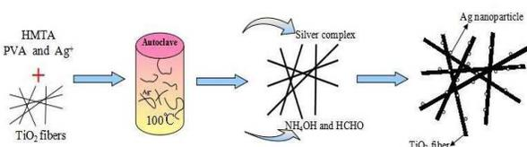
Scheme 1: The proposed schematic synthesis process to form Ag/TiO<sub>2</sub> nanoheterostructures by the solvothermal reducing reaction in HMTA solvent
