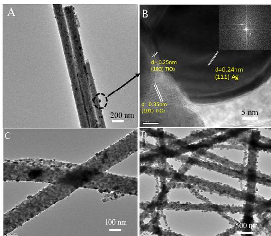
Fig. 3: The TEM image of Ag/ $\text{TiO}_2$  (A) and (B) the HRTEM for the specific area of the TEM in black circle (Inset part in Fig. 3B is the selected area Fourier Transform (FFT) from the HRTEM of silver particles), C and D were the TEM images of Ag/ $\text{TiO}_2$  samples, which prepared by 0.01 M and 0.05 M  $\text{AgNO}_3$  solutions respectively.
