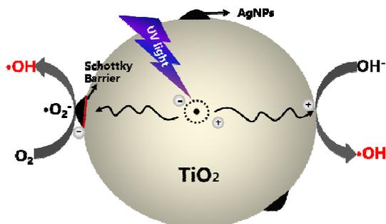
Scheme 2: Proposed mechanism of photo-generated charge separation and migration process in the Ag/TiO<sub>2</sub> nanoheterostructures under UV light
