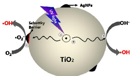
The proposed mechanism of photo-generated charge separation and migration process in the Ag/TiO<sub>2</sub> nanoheterostructures under UV light
