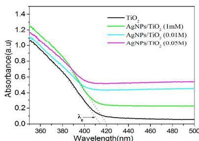
Fig. 4 UV-visible diffuse reflectance spectra of the  $\text{TiO}_2$  and Ag/ $\text{TiO}_2$  samples in the range of 350-500 nm
