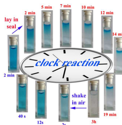
Fig. 6. Schematic representation of the “clock reaction” catalyzed by \text{Cu}_{1.8}\text{S} , that is, blue color fading and regeneration of MB.
