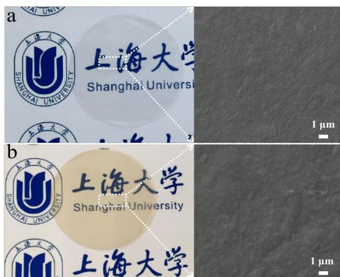
**Figure 2.** Digital images (left) and SEM images (right) of ONC film (a) and CDs/ONC composite film (b).
