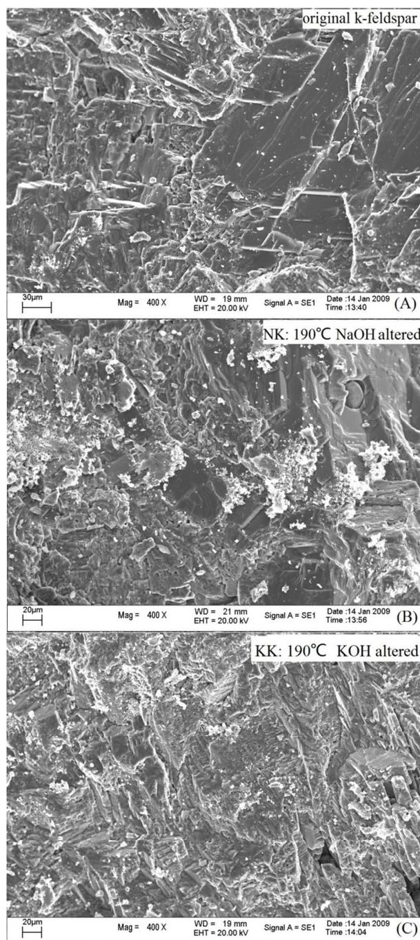
**Fig. 1 (A)-(C)** SEM of K-feldspar surface: (A) Original K-feldspar (OK); (B) NaOH-altered K-feldspar at 190 °C (NK); (C) KOH-altered K-feldspar at 190 °C (KK).
