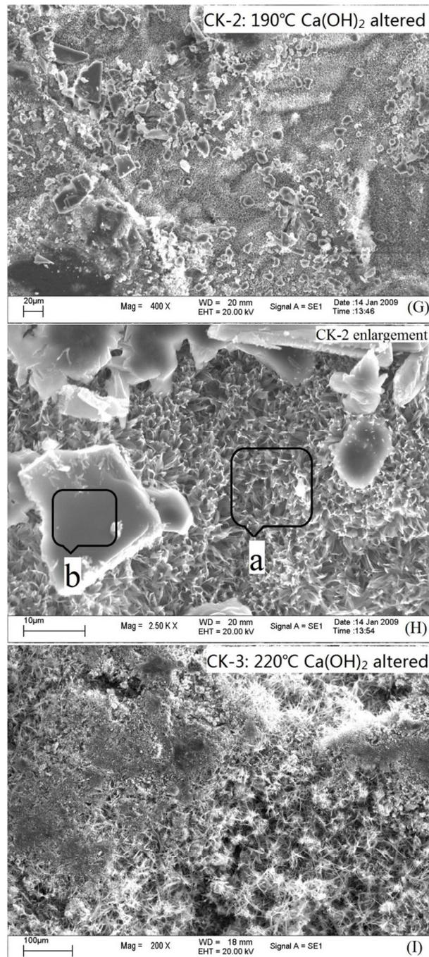
**Fig. 1 (G)–(I)** SEM of K-feldspar surface: (G) Ca(OH)<sub>2</sub>-altered K-feldspar at 190 °C (CK-2); (H) Enlargement of CK-2 (CK-2a, fiber; CK-2b, block); (I) Ca(OH)<sub>2</sub>-altered K-feldspar at 220 °C (CK-3).
