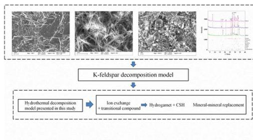
For the first time, a transitional compound  $[Ca^{2+} \equiv 2AlSi_3O_8 \equiv xOH^-]$  was observed for K-feldspar hydrothermal alkaline decomposition, and a model was presented.
