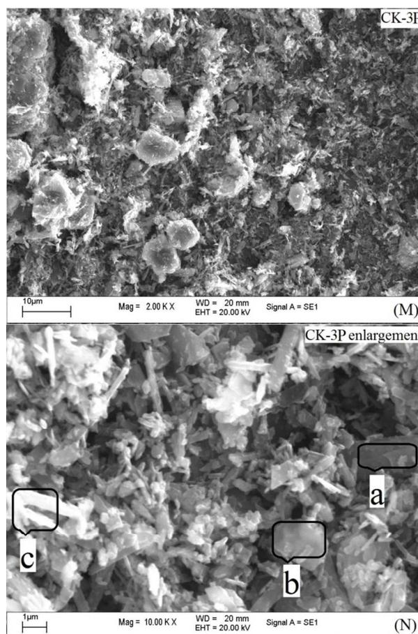
**Fig. 1 (M)-(N)** SEM of K-feldspar surface: (M) CK-3P (white precipitation in the filtrate of CK-3); (N) Enlargement of CK-3P (CK-3Pa, bar; CK-3Pb, sphere; CK-3Pc, needle).
