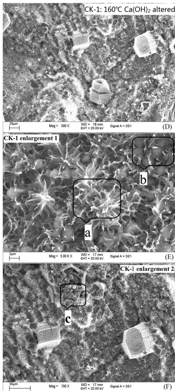
**Fig. 1 (D)–(F)** SEM of K-feldspar surface: (D) Ca(OH)<sub>2</sub>-altered K-feldspar at 160 °C (CK-1); (E) Enlargement part one of CK-1 (CK-1a, fiber; CK-1b, spherule); (F) Enlargement part two of CK-1 (CK-1c, polyhedron).
