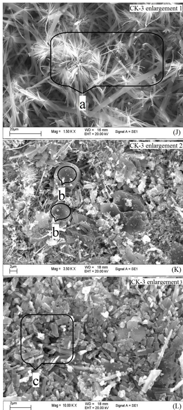
**Fig. 1 (J)-(L)** SEM of K-feldspar surface: (J) Enlargement part one of CK-3 (CK-3a, fiber); (K) Enlargement part two of CK-3 (CK-1b, octahedron); (L) Enlargement part three of CK-3 (CK-3c, bar).
