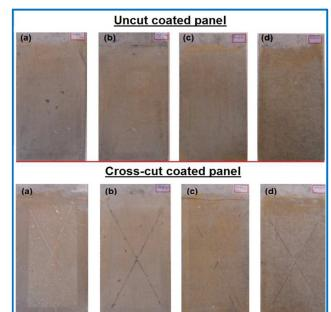
Fig. 6Corrosion showing on coating plates after 168 h with sequence - (a) succinic, (b) adipic, (c) suberic, (d) sebacic acid.
