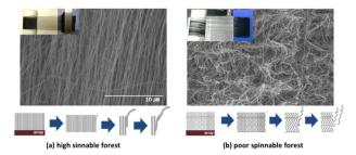
**Figure 6.** SEM images of the spinnable fibers responsible for the waviness of the CNT arrays: (a) straight arrays and (b) wavy arrays.
