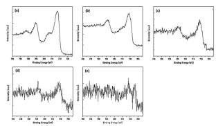
**Figure 5. Fe 2p** XPS spectra of substrates after CNTs were grown using  $[xFeCl_3:(1-x)FeCl_2]$  catalysts with various values of *x*: (a) x = 0, (b) x = 0.3, (c) x = 0.5, (d) x = 0.7, and (e) x = 1.
