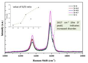
**Figure 3.** Raman spectra of CNTs prepared using  $[xFeCl_3:(1-x)FeCl_2]$  catalysts with various values of x (inset: change of the  $I_G/I_D$  ratio, where  $I_G$  and  $I_D$  represent the intensities of the G- and D-band, respectively).
