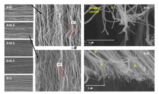
**Figure 1.** SEM images of the effect of catalyst composition  $[xFeCl_3:(1-x)FeCl_2]$ : (a),(f) x = 0; (b),(g) x = 0.3; (c) x = 0.5; (d) x = 0.7; and (e) x = 1.
