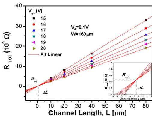
Fig. 5. Contact resistance of the coplanar homojunction a-IGZO TFTs with UV irradiated source/drain region was estimated by the transmission line method (TLM). The inset presents a magnified view in the small channel length region.
