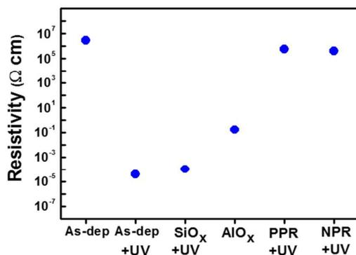
Fig. 3. Resistivity of a-IGZO films after UV irradiation through various UV shielding materials. UV light was irradiated for 3hrs after formation of a shielding layer with  $\text{SiO}_2$  (100 nm),  $\text{Al}_2\text{O}_3$  (100 nm), and PR (1.8  $\mu\text{m}$  PPR, NPR) on an a-IGZO thin film.
