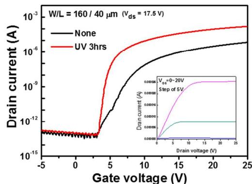
Fig. 4. Transfer characteristics of coplanar homojunction a-IGZO TFTs without and with  $n^+$  doping by UV irradiation of the source/drain region for 3 hrs. The channel width and length were fixed at 160  $\mu\text{m}$  and 40  $\mu\text{m}$ , respectively. The inset shows output characteristics of the a-IGZO TFT, which do not show any current crowding.
