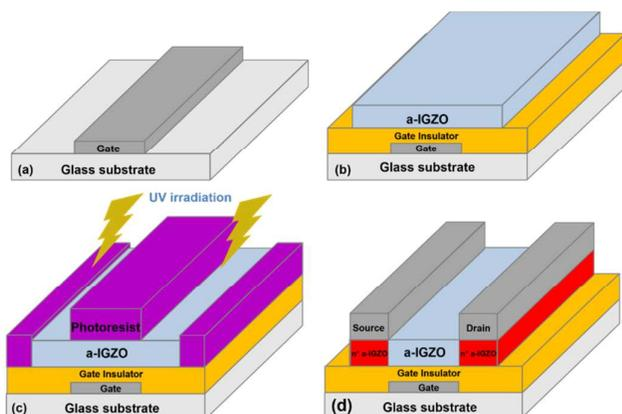
Fig. 1. A schematic representation of the fabrication process for coplanar homojunction a-IGZO TFTs: (a) gate metal deposition and patterning, (b) gate insulator and a-IGZO film deposition and patterning, (c) PR UV mask layer patterning followed by UV irradiation to form an n<sup>+</sup> a-IGZO region, and (d) source and drain formation using a lift-off method. The channel width (W) and length (L) are 160 μm and 40 μm, respectively.
