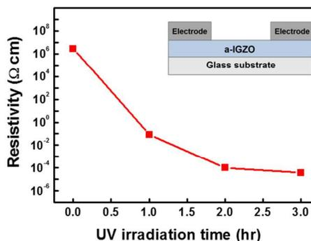
Fig. 2. Resistivity of a-IGZO films as a function of UV irradiation time. The resistivity of the as-deposited a-IGZO film was as high as  $2.71 \times 10^6 \Omega\cdot\text{cm}$ . After UV-irradiation for 3 hrs, the resistivity of the a-IGZO film dropped to  $3.76 \times 10^{-5} \Omega\cdot\text{cm}$ , which is similar to the level of typical transparent ITO electrodes ( $10^{-4}$ – $10^{-5} \Omega\cdot\text{cm}$ ).
