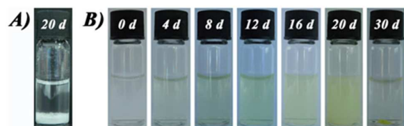
Figure 1. (A) Visual observation of the white precipitate at pH 2.0 after 20 days of incubation and (B) the solution evolution vs. time at pH 10.0 after dissolving Fmoc-5 in a HFIP/water mixture.
