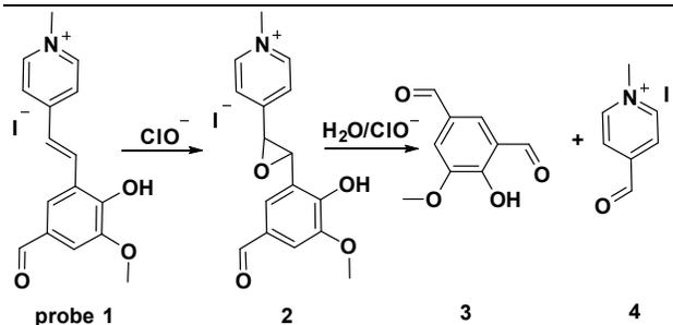
**Scheme 2.** Proposed detection mechanism of probe **1** towards HClO.
