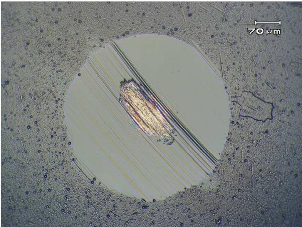
**Fig. 5** Surface topography of the worn surface on the flat under different temperatures
