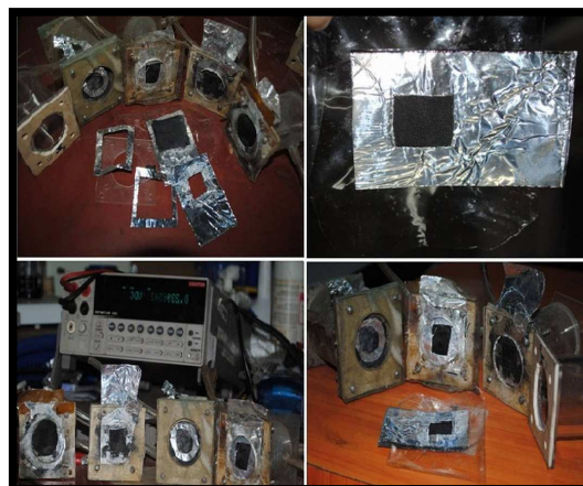
Fig 15: Membrane electrode assembly (MEA) in single chambered MFCs
