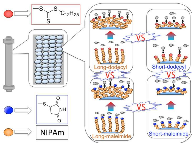
Even using the same homo poly(*N*-isopropylacrylamide) immobilized silica beads as stationary phases, terminal functional group and chain length significantly affected temperature-dependent elution behavior of steroids.
