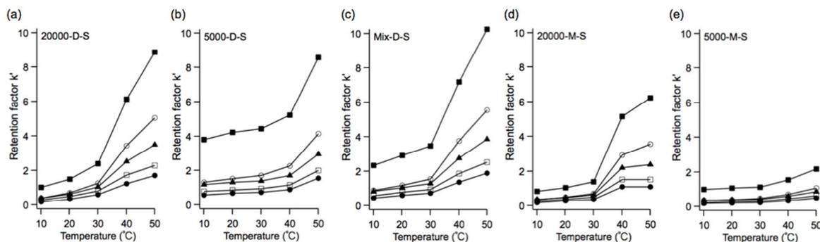
Fig. 5 Temperature-dependent retention factors of five steroids on (a) 20000-D-S, (b) 5000-D-S, (c) Mix-D-S, (d) 20000-M-S, and (e) 5000-M-S HPLC columns: (●) hydrocortisone, (□) prednisolone, (▲) dexamethasone, (○) hydrocortisone acetate, and (■) testosterone.
