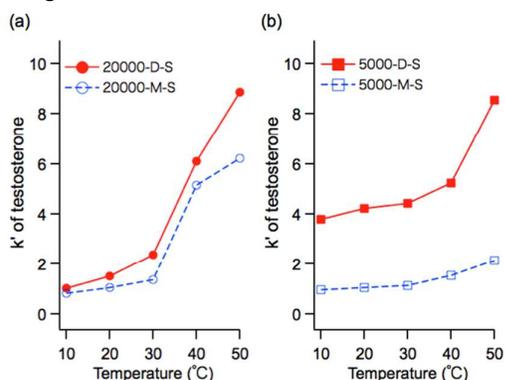
**Fig. 7** Temperature-dependent retention factors of testosterone on PNIPAAm-grafted silica columns with a molecular weight of (a) 20000 g/mol, and (b) 5000 g/mol.
