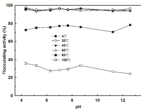
Fig. 7. The pH receptivity and thermostability of MBF412.
