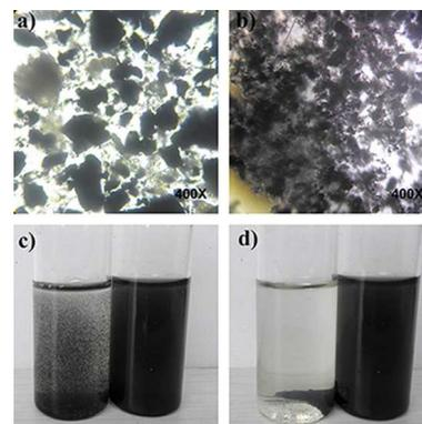
**Fig. 9.** Image-analysis of the wastewater: a): Polluted particles before sedimentation examined under a microscope; b): Polluted particles with  $\text{CaCl}_2$  and bioflocculant after sedimentation examined under a microscope; c): Polluted particles during sedimentation; d): Polluted particles after sedimentation.
