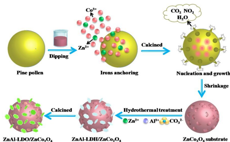
2 3 Fig. 8. Schematic illustration of the synthesis of pollen-like \text{ZnAl-LDH/ZnCo}_2\text{O}_4 and its derived metal oxides
