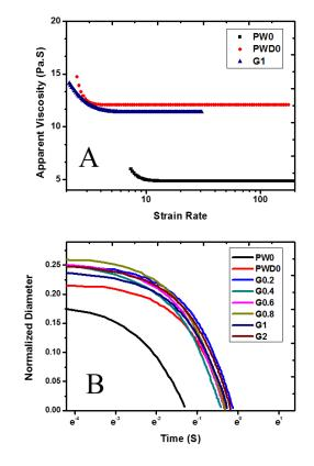
Fig. 3 A) Apparent viscosity vs. strain rate of PWO, PWDO, and G1 samples, and B) normalized diameter vs. time graph of all samples.
