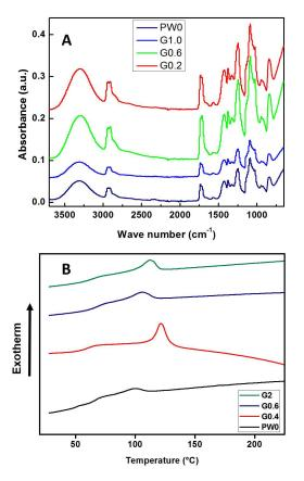
Figure 6 A) FT-IR spectra of selected sample and B) DSC analysis of selected as spun mats at the cooling region.
