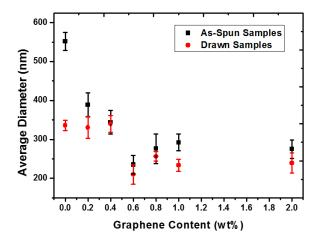
Fig. 8 Average diameter of sample fibers at as-spun and after drawing during UTM analysis states, respectively versus the incorporated graphene content.
