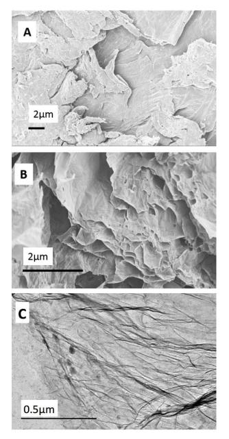
Fig. 2 SEM images of A) GO, B) rGO, and C) TEM image of rGO.
