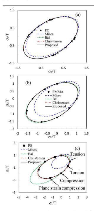
**Fig.2** Comparison between the experiment data with four forms of equivalent stress in plane stress space, i.e., Mises, Bai, Christensen and the proposed form: (a) PC, (b) PMMA ( $@60^{\circ}C$ ), (c) PS ( $@90^{\circ}C$ ). The experiment data of PMMA and PS are from the literature.<sup>27</sup>
