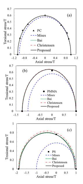
**Fig.1** Comparison between the experiment data with four forms of equivalent stress under combined axial-torsional condition, i.e., Mises, Bai, Christensen and the proposed form: (a) PC, (b) PMMA ( $@60^{\circ}$ C), (c) PS ( $@90^{\circ}$ C). The experiment data of PMMA and PS are from the literature.<sup>27</sup>
