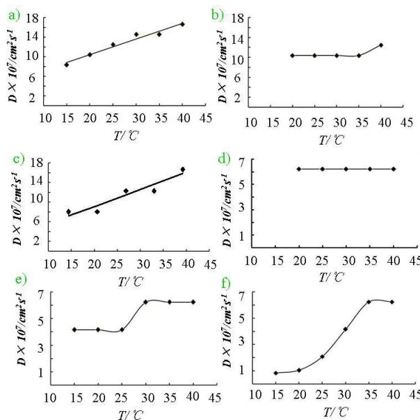
**Fig.5** Effect of temperature on the permeation of NaCl through different membrane(s) with PAAC or PAAM switches. a) the Virgin N6 membrane. b) the N6-i-PAAC membrane ( $Y_{PAAC}=5.47\%$ ). c) the N6-i-PAAM membrane ( $Y_{PAAM}=6.43\%$ ). d) Two virgin N6 membranes. e) the C-M coupling membranes. f) the M-C coupling membranes ( $Y_{PAAC}=5.47\%$  and  $Y_{PAAM}=6.43\%$ ).
