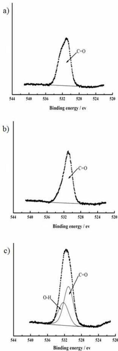
**Fig.3** XPS O1s core-level spectra of a) the virgin N6 membrane, b) the immobilizing-PAAM membrane, and c) the immobilizing-PAAC membrane.
