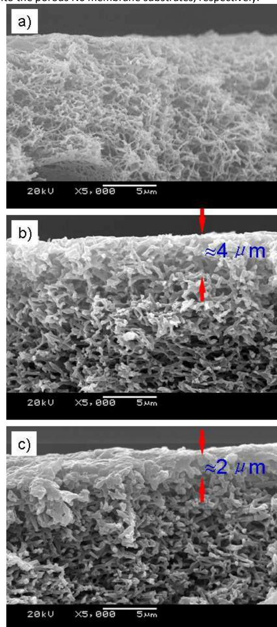
**Fig.4** SEM micrographs of the cross sections of a) the virgin N6 membrane, b) the N6-*i*-PAAM membrane ( $Y_{PAAM}=6.43\%$ ), c) the N6-*i*-PAAC membrane ( $Y_{PAAC}=5.47\%$ ). Scale bar 5μm.
