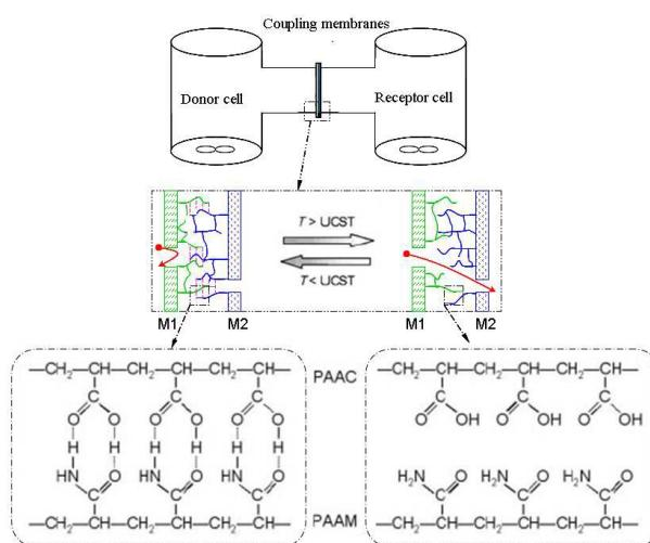
**Fig.1** Schematic illustration of the concept of the proposed positively thermoresponsive switch membranes.
