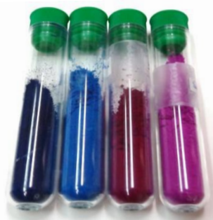
Figure 2. Resulting sepiolite pigment: MB_{ss} , MB_{as} , MR_{ss} , MR_{as} (from left to right)
