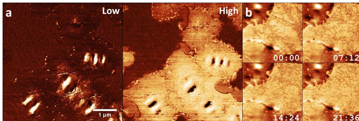
Figure 7. (a) Phase images taken at low and high tapping force exhibit a difference in contrast. The images were taken at the same location as in Fig. 4c. (b) Topography images of the para
