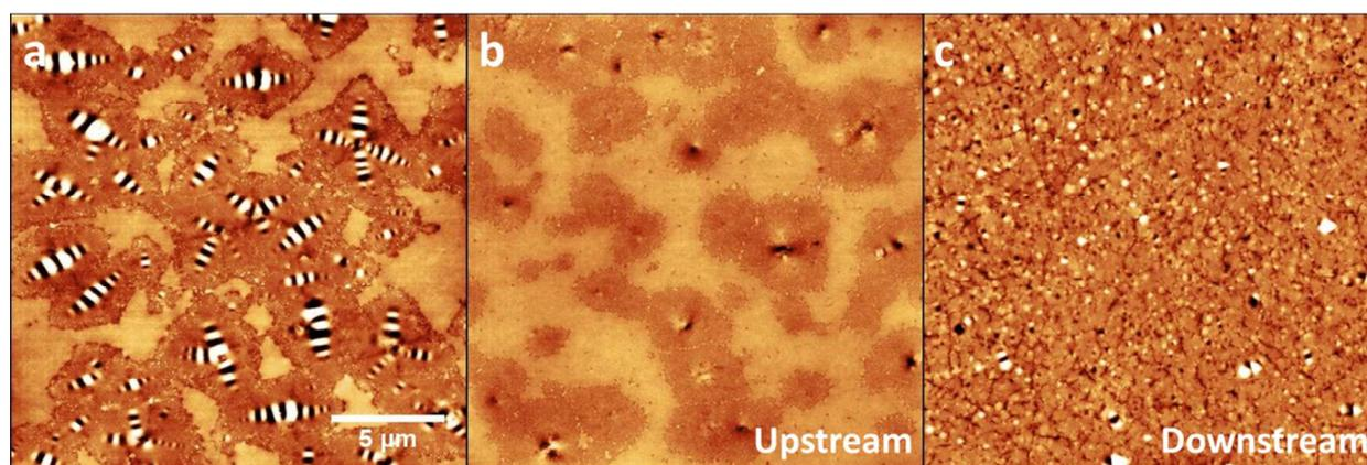
Figure 6. AFM topography images of (a) typical “bee” structures and (b, c) different textures that resulted from flow during cooling. The imaged areas are (b) upstream or (c) downstream of the flow. Images (a) and (b) are of two locations only 2 mm apart on the same specimen. Height scale is 20 nm and scale bar applies to all images.
