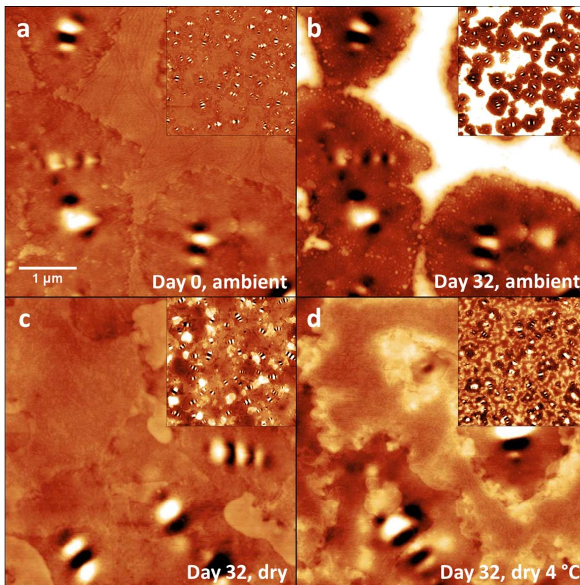
Figure 4. AFM topography images show the effect of storage conditions on the evolution of bee-like structures after 32 days. The samples were stored under (a, b) ambient temperature and humidity (22 °C, 50% humidity), (c) room temperature in dry air, or (d) 4°C in dry air. Scale bar applies to all images, insets are 20 μm square areas, and the height scale for all images is 25 nm.
