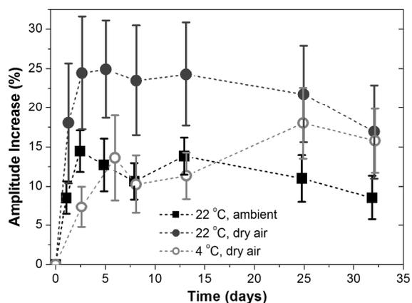
Figure 5. Change in amplitude the “bee” structures plotted as functions of time and storage conditions. Error bars are 5% confidence interval.
