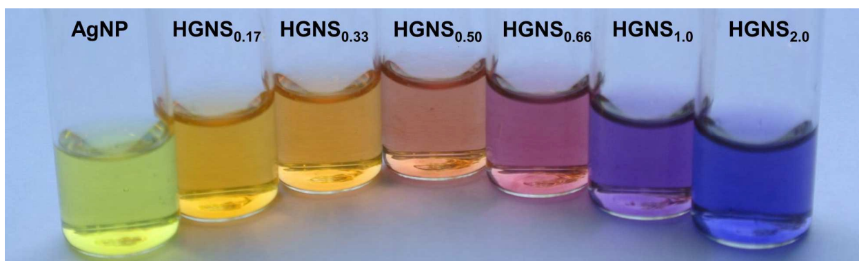
Fig. 3 Photograph of aqueous colloidal solution of silver nanospheres and different hollow gold nanostructures batches prepared with different molar ratios of gold to silver. The term 'HGNS x ' used in this article is to define the HGNS type in which 'x' represents the molar ratio of gold to silver.
