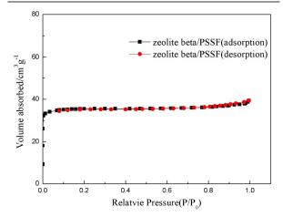
Fig. 4.  $N_{\rm 2}$  adsorption/desorption of the zeolite beta coating/PSSF composite at 77K.
