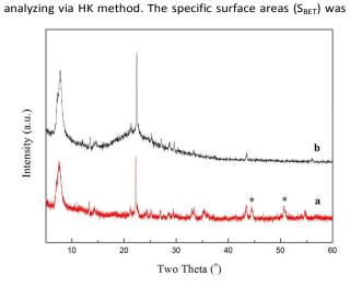
Fig. 3. X-ray diffraction patterns of different samples: (a) zeolite beta coating/PSSF composite; (b) samples deposited on the bottom of the autoclave.
