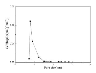
Fig. 5. Pore size distribution of the zeolite beta coating/PSSF composite.
