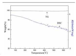
Fig. 6. TG-DSC curves of the zeolite beta coating/PSSF composite.
