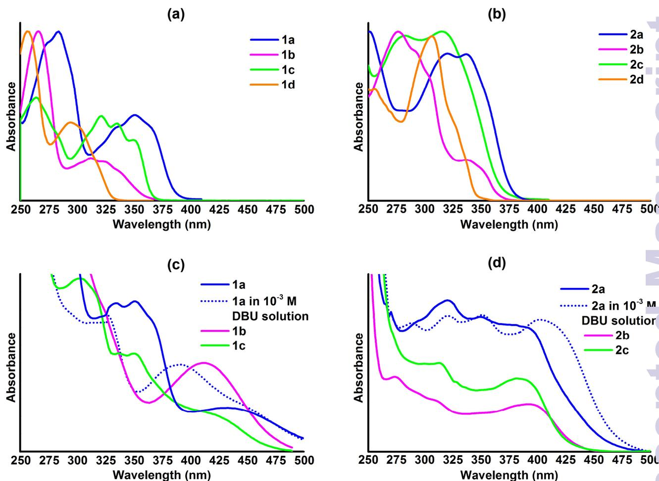
**Fig. 1** Steady-state absorption spectra at 298 K: **1a-d** (a) and **2a-d** (b) in methycyclohexane; **1a-c** (c) and **2a-c** (d) in  $10^{-4}$  M DBU solution in methycyclohexane
