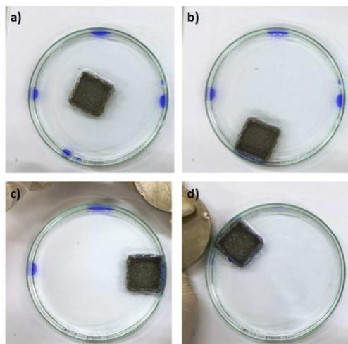
Fig. 7. a) Dye-colored water on the surface of the dichloromethane in a watch glass; b,c) subsequent removal of the little water by the magnetically driven the as-prepared device; d) Cleaned oil surface after the process.
