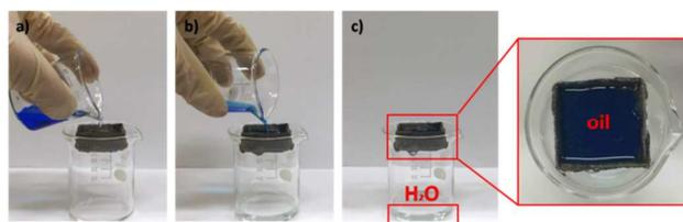
Fig. 4. The oil-water separation process: a) A mixture of water and blue-dyed oil was poured into the device. b) Water passed through the device, c) while oil was prevented from permeating into the hydrogel and remains in the device.
