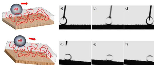
Fig. 3. The dynamic underwater oil adhesion measurement on as-prepared device surface: a-c) An oil droplet was applied to contact the surface and can be moved easily; d-f) The slant surface showed an ultralow affinity to the oil droplet.
