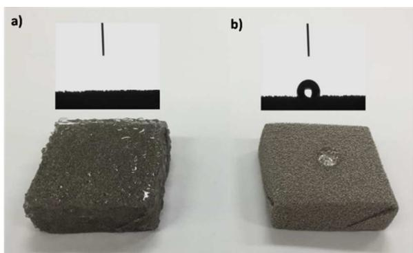
Fig. 2. CA and photographs of water droplets on different surfaces: a) PAM hydrogel coated nickel foam and b) bare nickel foam
