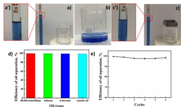
Fig. 5. The process a-c) of evaluating the separation efficiency of the dichloromethane-water mixture by as-prepared device; The magnification of a) and c) indicate the volumes in the pipette; d) Separation efficiency of the as-prepared device for different oil-water mixtures; e) Recycled experiments for separating oil from water by as-prepared device.
