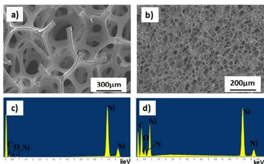
Fig. 1. SEM images of the nickel foam a) before and b) after modification by PAM hydrogel; the corresponding EDX patterns for c) bare nickel foam and d) modification by PAM hydrogel.
