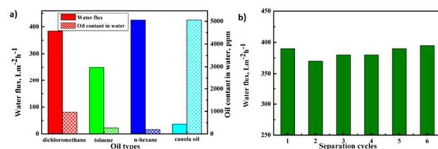
Fig. 6. Oil-water separation results of the as-prepared device. a) Oil content and the water flux after permeating a series of immiscible oil-water mixtures. b) Water flux for permeating oil-water mixture through the as-prepared device with different cycle index.
