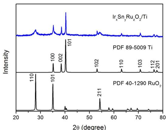
**Fig. 3** XRD pattern of the surface of the Ir<sub>x</sub>Sn<sub>y</sub>Ru<sub>z</sub>O<sub>2</sub>/Ti electrode.
