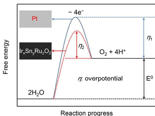
**Fig. 7** Qualitative reaction scheme for OER on Pt anode or  $\text{Ir}_x\text{Sn}_y\text{Ru}_z\text{O}_2/\text{Ti}$  anode.
