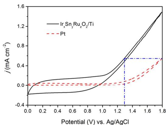
**Fig. 4** CV curves of OER on the Pt electrode and the Ir<sub>x</sub>Sn<sub>y</sub>Ru<sub>z</sub>O<sub>2</sub>/Ti electrode.
