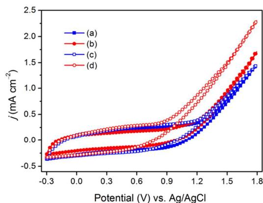
**Fig. 10** CV curves on the  $\text{Ir}_x\text{Sn}_y\text{Ru}_z\text{O}_2/\text{Ti}$  electrode with (a) or without (c) Nafion membrane in electrolytes and CV curves on the  $\text{Ir}_x\text{Sn}_y\text{Ru}_z\text{O}_2/\text{Ti}$  electrode with (b) or without (d) Nafion membrane in electrolytes containing  $0.05 \text{ mol L}^{-1} \text{ HCOO}^-$ . The measurements were performed in  $0.1 \text{ mol L}^{-1} \text{ KHCO}_3$  electrolyte after being bubbled with  $\text{CO}_2$  for 30 min.
