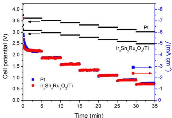
**Fig. 6** Current densities at different cell potentials when use the Pt electrode or the  $\text{Ir}_x\text{Sn}_y\text{Ru}_z\text{O}_2/\text{Ti}$  electrode as anode during the electrochemical reduction of  $\text{CO}_2$  in  $0.1 \text{ mol L}^{-1}$   $\text{KHCO}_3$  solution.
