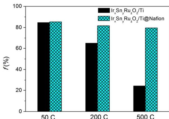
**Fig. 9** Variations in faradaic efficiency for producing formate with the charge passed when the anode is  $\text{Ir}_x\text{Sn}_y\text{Ru}_z\text{O}_2/\text{Ti}$  or  $\text{Ir}_x\text{Sn}_y\text{Ru}_z\text{O}_2/\text{Ti}@$ Nafion electrode.
