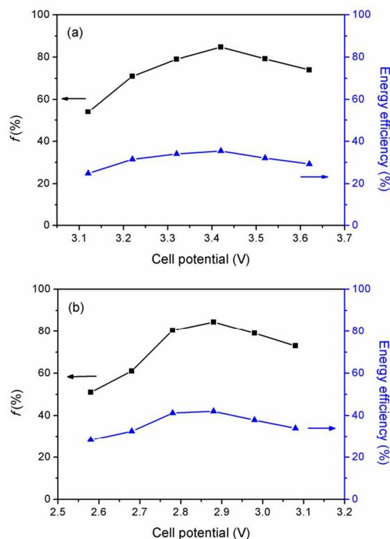
**Fig. 8** Variations of energy efficiency and faradaic efficiency for producing formate on the Sn electrode with the applied potential when using the Pt electrode (a) or the  $\text{Ir}_x\text{Sn}_y\text{Ru}_z\text{O}_2/\text{Ti}$  electrode (b) as the anode.
