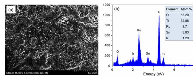
Fig. 2 SEM image (a) and EDS spectrum (b) of the surface of the Ir<sub>x</sub>Sn<sub>y</sub>Ru<sub>z</sub>O<sub>2</sub>/Ti electrode.
