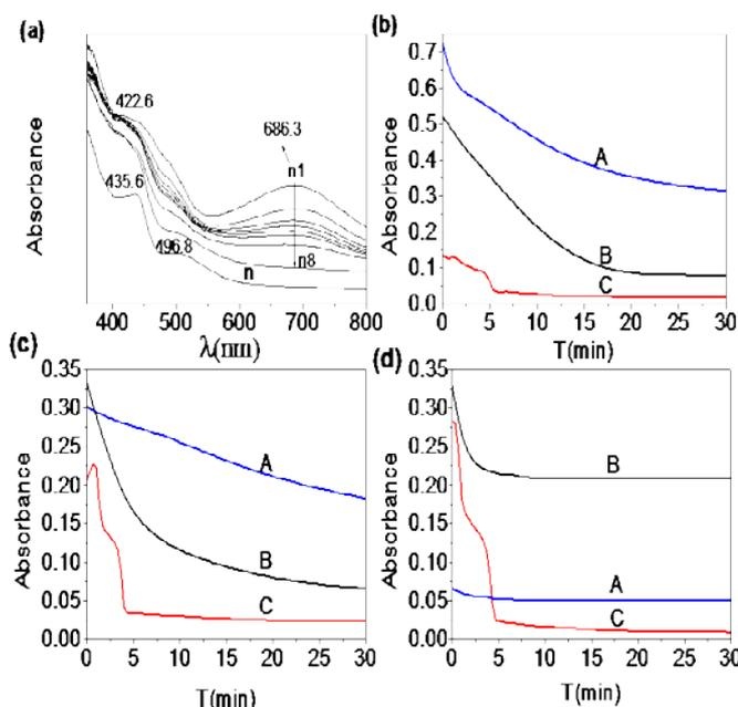
Fig. 2. (a) UV-vis spectra of [salen-Mn(III)](Cl), [salen-Mn(III)](Cl)+m-CPBA in CH<sub>2</sub>Cl<sub>2</sub> (0.1mM) in dependence of time (every 20mins from the top down n1-n6, n7, 6h, n8, 8h). (b-d) The changing curves of Mn<sup>V</sup>=O absorbance of [salen-Mn(III)](Cl), [salen-Mn(III)](NO<sub>3</sub>) and [salen-Mn(III)](BF<sub>4</sub>) with time in A: DCM, B: CH<sub>3</sub>CN, C: DMF.
