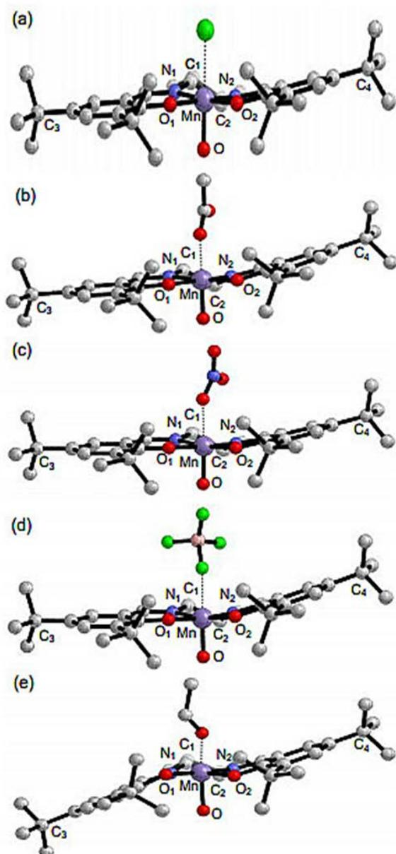
Fig. 1. The optimized structures of  $[\text{Mn}^{\text{V}}=\text{O}(\text{salen})][\text{X}]$ , (a)  $\text{X}^- = \text{Cl}^-$ , (b)  $\text{X}^- = \text{OAc}^-$ , (c)  $\text{X}^- = \text{NO}_3^-$ , (d)  $\text{X}^- = \text{BF}_4^-$ , (e)  $\text{X}^- = \text{CH}_3\text{CH}_2\text{O}^-$
