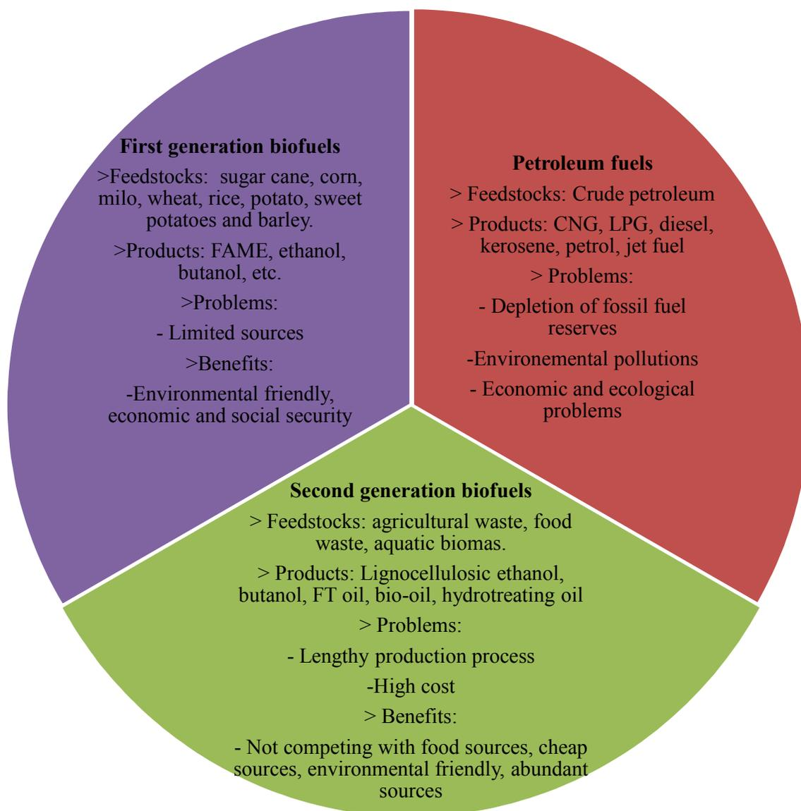
Fig. 4 Comparison of the petroleum refinery products, first and second generation of the biofuels production <sup>47</sup>.
