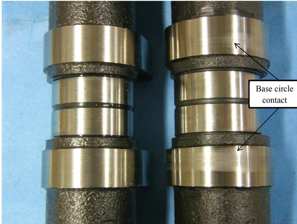
Fig. 12 Exhaust cam lobes base circle details for cylinder 3, E0 cam lobe on Left, E15 cam lobe on Right<sup>180</sup>.
