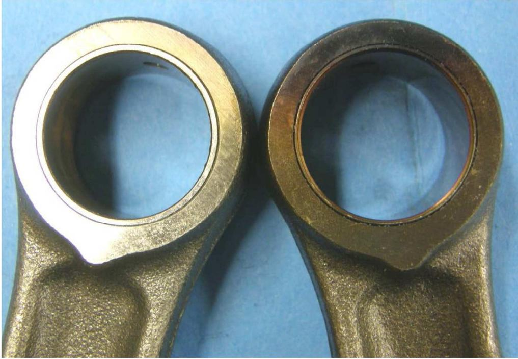
Fig. 11 Connecting rod carbon deposit comparison for cylinder 2, E0 connecting rod on Left,
