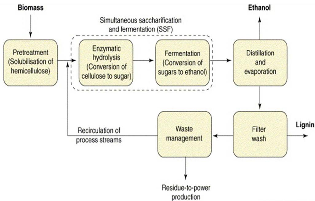
Fig. 5 Production process for bioethanol from lignocellulosic biomass<sup>51</sup>.
