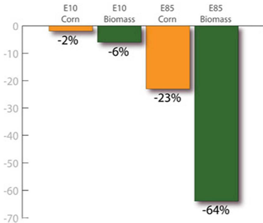
Fig. 3 Reduction of Greenhouse Gas (GHG) emissions from cellulosic bioethanol and corn-derived bioethanol blends <sup>50</sup>.
