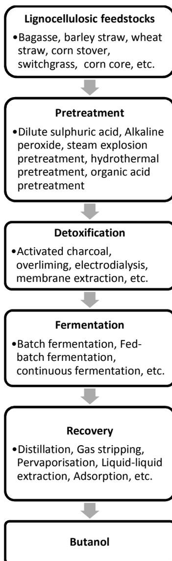
Fig. 6 Production process for biobutanol from lignocellulosic feedstocks<sup>72, 73</sup>.
