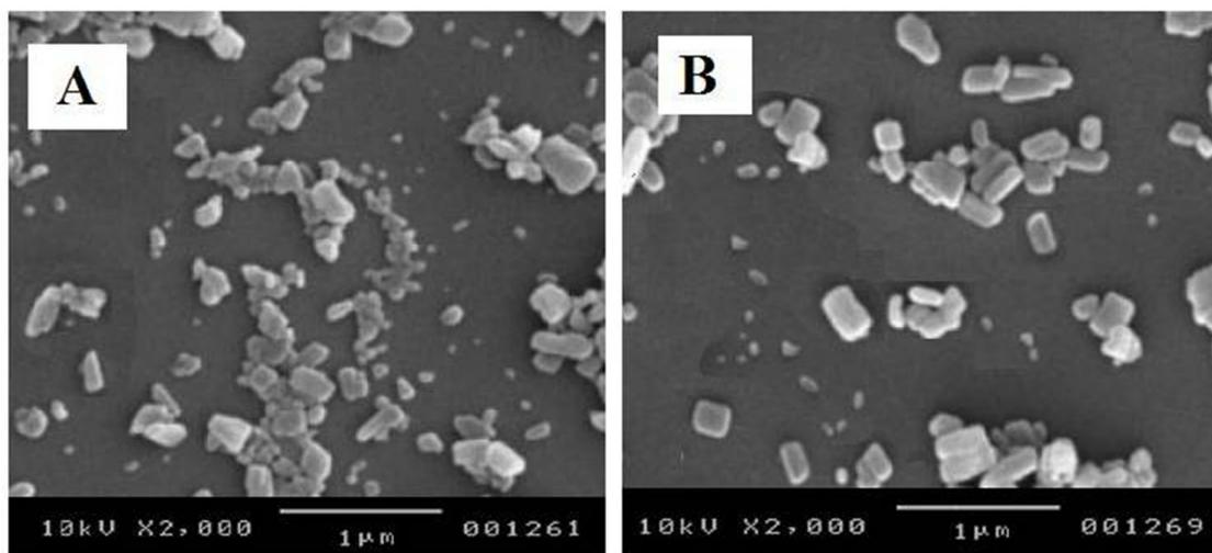
**Figure 8: SEM of glibenclamide nanoparticles: (A) formulation GD-H0.3d; (B) formulation GD-L0.4f.**
