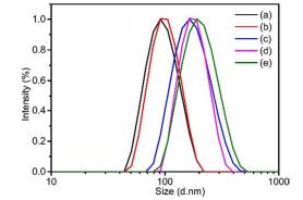
**Figure 5** Particle sizes and distributions of (a) FPU20, (b) FSPU3, (c) FSPU6, (d) FSPU8 and (e) FSPU10 dispersions.
