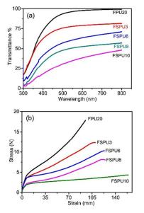
Figure 8 (a) UV-vis results and (b) stress-strain curves of FPU20, FSPU3, FSPU6, FSPU8 and FSPU10
