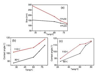
**Figure 10** Average particle sizes of (a) FPU20 and FPU30 hybrid films at different polymerization temperature; Water contact angles and polymerization temperature profiles of (b) FPU20 and (c) FPU30 hybrid films, both films were dried at 80 °C and 110 °C.
