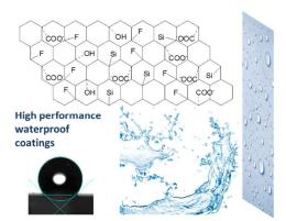
Novel waterborne polyurethane containing fluorine and siloxane (FSPU) for excellent thermal performance, waterproof and mechanical properties.
