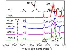
Figure 1 FTIR spectra of IPDI, FMA, WPU, FPU30, SPU10 and FSPU8
