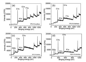
**Figure 3** XPS spectra of (a) surface of FPU10, (b) interface of FPU10, (c) interface of SPU10 and (d) interface of FSPU10.
