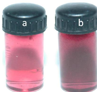
Fig 1. Photographs of a) pure cobalt and b) MWCNTs dispersed in cobalt solution
