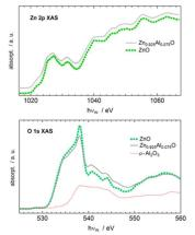
Fig. 4. Zn 2p (top panel) and O 1s (lower panel) X-ray absorption of the ZnO (solid line) and the  $Zn_{0.925}Al_{0.075}O$  (dashed line) nanocrystals.
