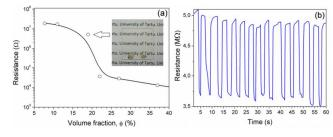
**Fig. 6.** Percolation behaviour (a) and piezoresistive performance (b) of  $Zn_{0.925}Al_{0.075}O/PDMS$  composite.
