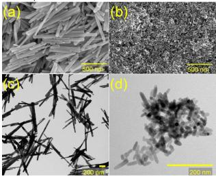
Fig. 2. SEM images for ZnO (a) and  $Zn_{0.85}AI_{0.15}O$  (b) and TEM for ZnO (c) and  $Zn_{0.85}AI_{0.15}O$  (d).
