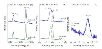
Fig. 3. XPS spectra measured from Zn 2p, O 1s, Al 2p and valence band region of ZnO and  $Zn_{0.925}Al_{0.075}O$  nanocrystals.
