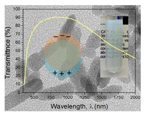
Ethanol solvothermal method derives plasmonic Al doped ZnO nanocrystals suitable for advanced applications.
