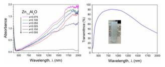
**Fig. 5.** Left panel: UV-NIR absorption spectra (Kubelka–Munk function) for different AZO samples. Right panel: the optical transmittance spectrum of  $Zn_{0.85}Al_{0.15}O$  colloid solution in a mixture of butylamine (20%) and dichlormethane (80%). The inset shows a photograph of the concentrated stock colloid (15 mg/ml), which was 10 times diluted for the transmittance measurement.
