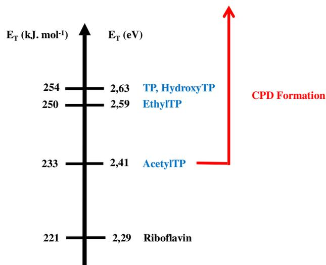
Figure 5. Lower limit threshold of a photosensitizer triplet state energy (in  $\text{kJ.mol}^{-1}$  and eV) for CPD formation (from estimated values for TTET).
