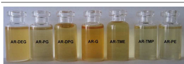
Figure 4. The color of the alkyd resins synthesized from glycolizate based on waste PET.
