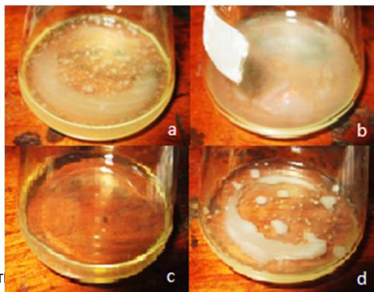
**Figure 8** (a) Bacterial suspension used for filtration (b) Filtrate of GAC filter (c) Filtrate of HAP filter (d) Filtrate of HAP/GAC filter
