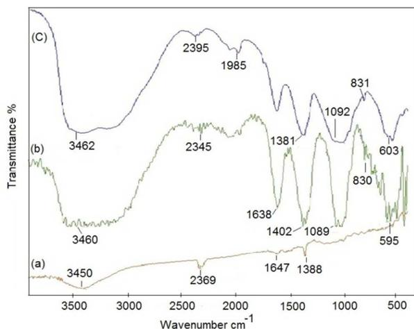
**Figure 1.** FT-IR spectra of pure (a) GAC (b) HAP/GAC (c) pure HAP
