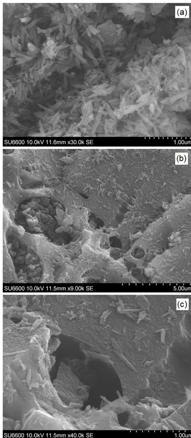
**Figure 2.** SEM images of (a) pure nano Hydroxyapatite (HAP) (b) HAP/GAC low magnification (c) HAP/GAC high magnification
