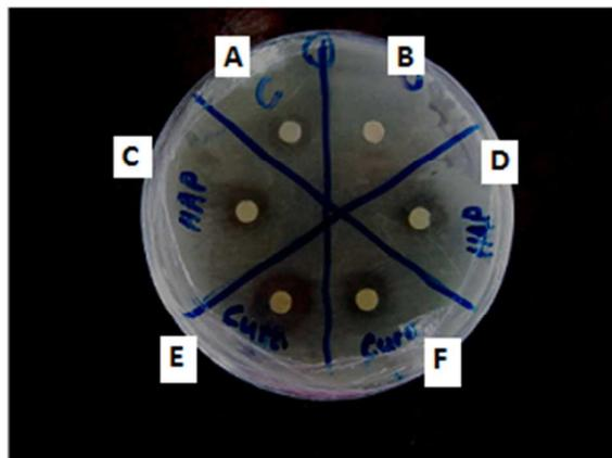
**Figure 7.** Inhibitions zones. A – Positive Control (1.2 cm); B – Negative Control (0.0 cm); C,D – HAP (1.2 cm, 1.1 cm); E,F – HAP coated with Curcumin (1.5 cm, 1.3 cm)
