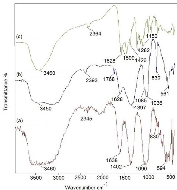
**Figure 5** . Comparison of FT-IR spectra of (a) HAP coated GAC (b) HAP-Curcumin bi-coated GAC (c) Curcumin
