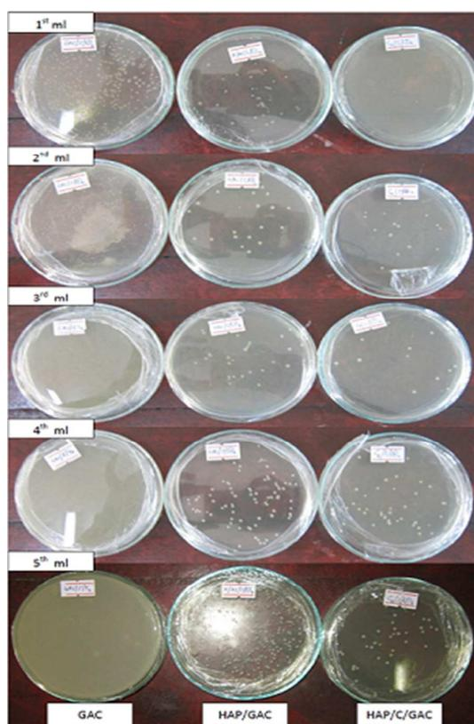
**Figure 10.** Comparison of the effects of HAP/GAC and HAP/C/GAC filters with the GAC filter.
