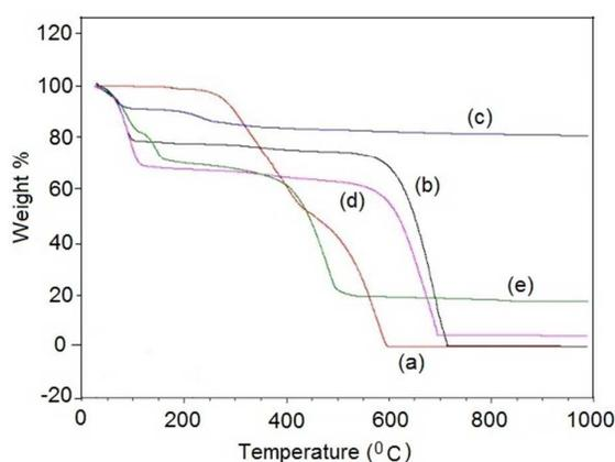
**Figure 6** . Comparison of TGA curves obtained for (a) Curcumin (b) GAC (c) HAP (d) HAP/Curcumin/GAC (e) HAP/GAC
