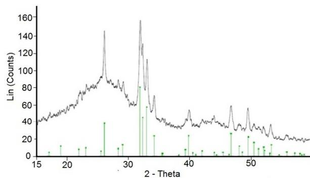
**Figure 3.** Comparison of XRD pattern of HAP/GAC with standard HAP
