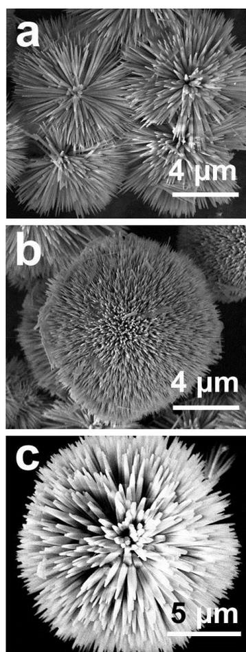
**Fig. 1** SEM images of the  $\text{Co}_3\text{O}_4$  precursors synthesized at 150  $^\circ\text{C}$  for different hydrothermal reaction times: (a) CP-A, 0.5 h; (b) CP-B, 1 h; (c) CP-C, 6 h.
