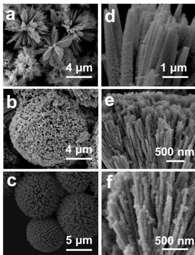
**Fig. 3** SEM images of the urchin-like  $\text{Co}_3\text{O}_4$  at different resolutions: (a, d)  $\text{Co}_3\text{O}_4$ -A; (b, e)  $\text{Co}_3\text{O}_4$ -B and (c, f)  $\text{Co}_3\text{O}_4$ -C.
