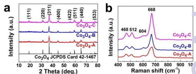
**Fig. 2** (a) XRD patterns of  $\text{Co}_3\text{O}_4$ -A,  $\text{Co}_3\text{O}_4$ -B,  $\text{Co}_3\text{O}_4$ -C and standard of  $\text{Co}_3\text{O}_4$  from JCPDS card 42-1467; (b) Raman spectrum of  $\text{Co}_3\text{O}_4$ -A,  $\text{Co}_3\text{O}_4$ -B,  $\text{Co}_3\text{O}_4$ -C.
