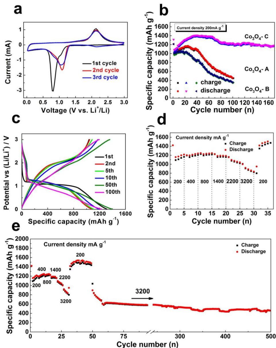
**Fig. 6** (a) CV curves of Co<sub>3</sub>O<sub>4</sub>-C at a scan rate of 0.1 mV s<sup>-1</sup> for the first three cycles; (b) cycling performance of Co<sub>3</sub>O<sub>4</sub>-A, Co<sub>3</sub>O<sub>4</sub>-B and Co<sub>3</sub>O<sub>4</sub>-C electrode at 200 mA g<sup>-1</sup>; (c) charge-discharge curves for selected cycles of 3D hierarchical urchin-like Co<sub>3</sub>O<sub>4</sub> electrode at 200 mA g<sup>-1</sup>; (d, e) rate performance of Co<sub>3</sub>O<sub>4</sub>-C electrode.
