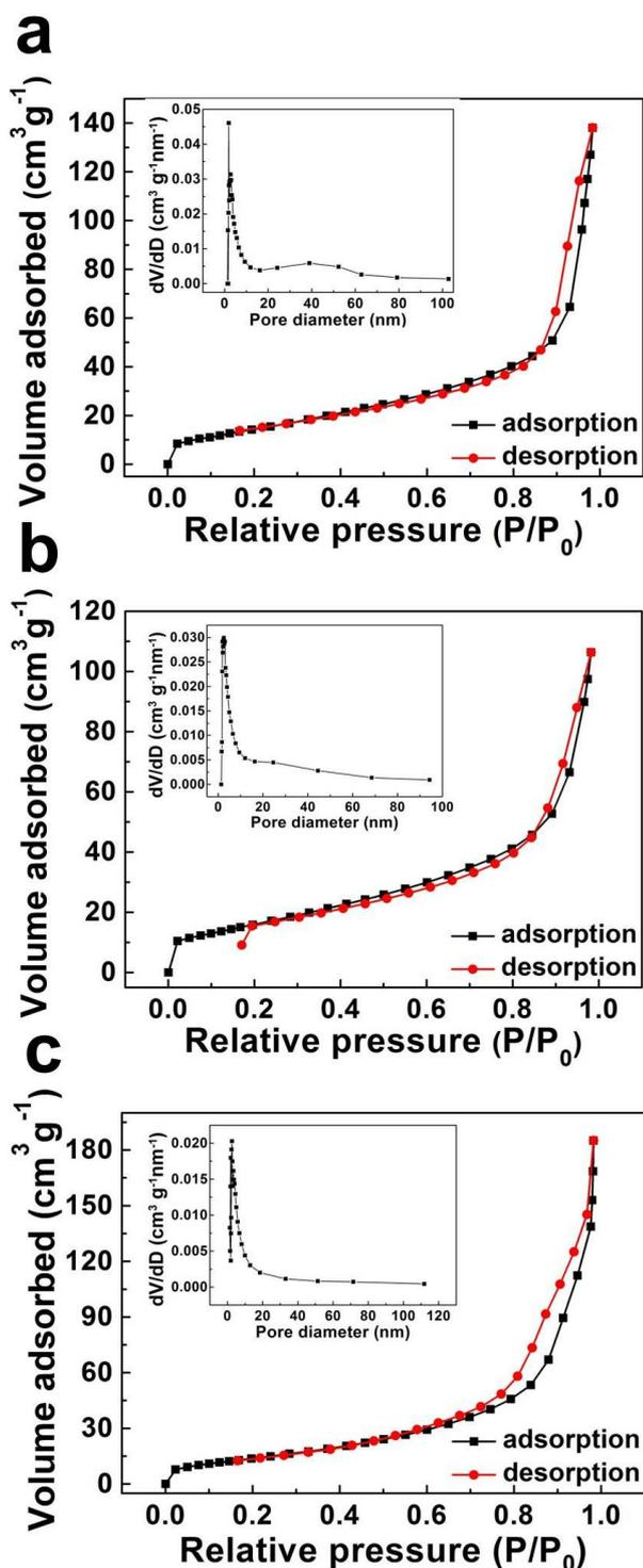
Fig. 5 Nitrogen adsorption-desorption isotherms and BJH pore size distribution plots (insets) of (a)  $\text{Co}_3\text{O}_4\text{-A}$ , (b)  $\text{Co}_3\text{O}_4\text{-B}$  and (c)  $\text{Co}_3\text{O}_4\text{-C}$ .
