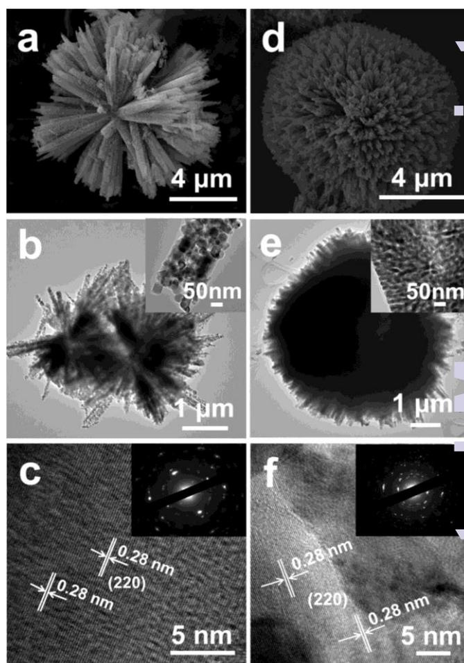
**Fig. 4** SEM images of (a)  $\text{Co}_3\text{O}_4$ -A and (d)  $\text{Co}_3\text{O}_4$ -C; TEM images of (b)  $\text{Co}_3\text{O}_4$ -A and (e)  $\text{Co}_3\text{O}_4$ -C; HR-TEM images and the corresponding SAED patterns (insets) of (c)  $\text{Co}_3\text{O}_4$ -A and (f)  $\text{Co}_3\text{O}_4$ -C.
