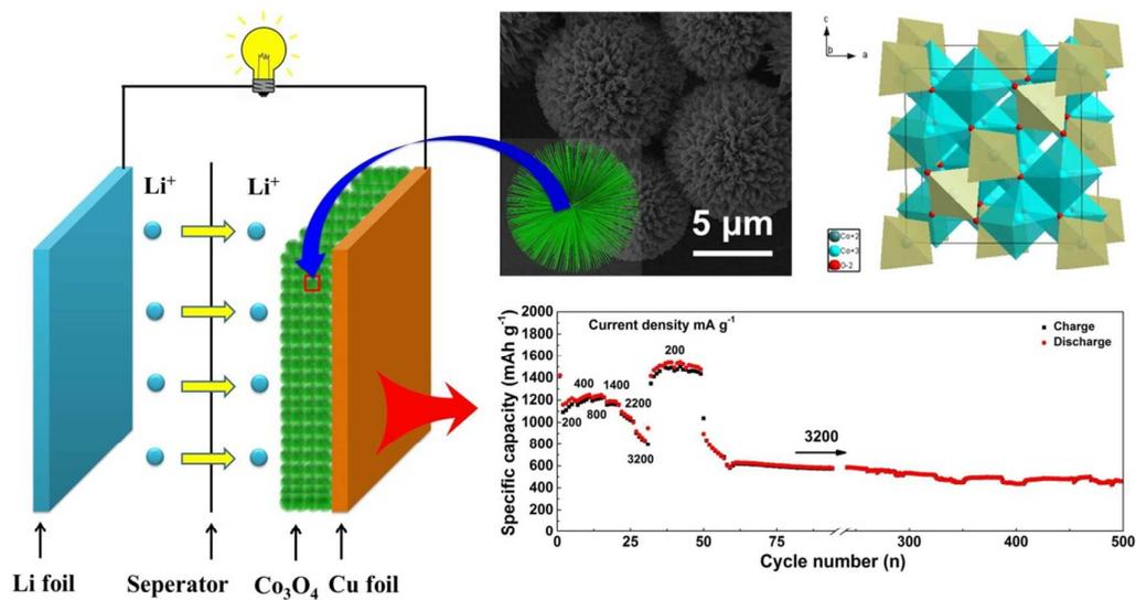
3D hierarchical  $\text{Co}_3\text{O}_4$  microspheres are fabricated by a very facile and green hydrothermal process. When applied in LIBs anode, the 3D hierarchical urchin-like  $\text{Co}_3\text{O}_4$  exhibits high reversible discharge capacity, excellent rate capability and good cycling performance.
