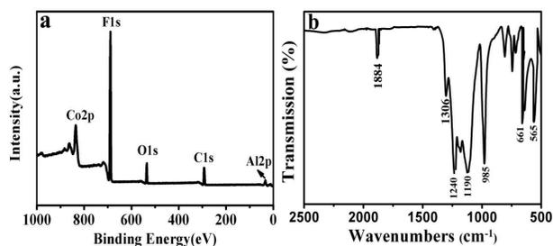
Fig. 3 XPS survey (a) and FT-IR (b) of  $\text{Co}_3\text{O}_4$  AAO growth super slippery surfaces
