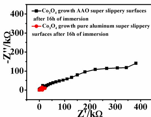
Fig. 8 Nyquist plots of  $Co_3O_4$  growth AAO and pure aluminium super slippery surfaces after immersion of 16h in 3.5% NaCl solution
