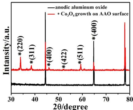
Fig. 2 X-ray diffraction of as-prepared AAO substrate and  $\text{Co}_3\text{O}_4$  growth AAO super slippery surfaces
