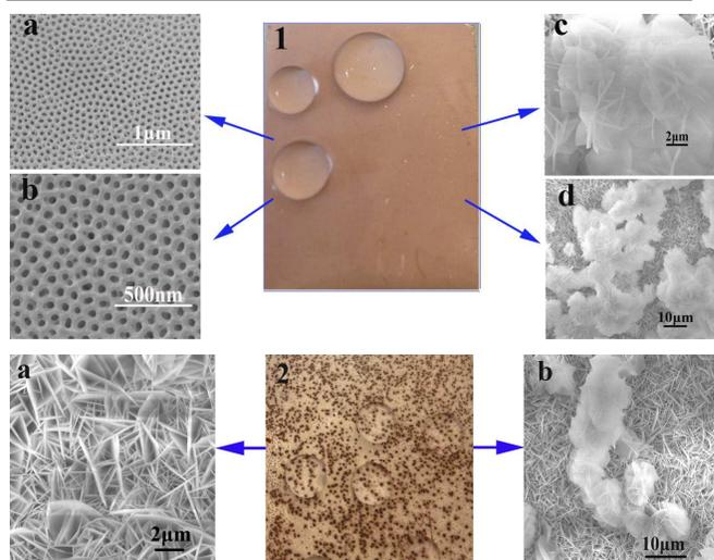
Fig. 1 SEM image of porous anodic aluminium oxide (1a-b);  $\text{Co}_3\text{O}_4$  growth on AAO (1c-d)
