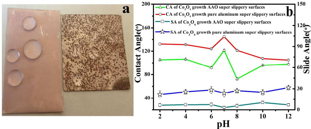
Fig. 6 (a) Water on  $\text{Co}_3\text{O}_4$  growth AAO super slippery surfaces (left) and  $\text{Co}_3\text{O}_4$  growth pure aluminium super slippery surfaces (right); (b) Variation of contact angles and slide angles of different pH
