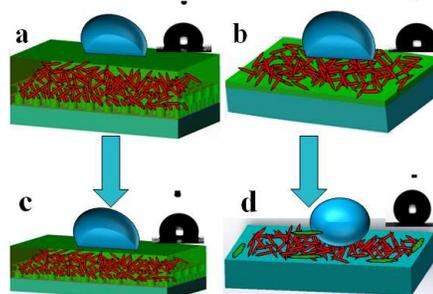
Fig. 4 Schematic showing porosity changes of  $\text{Co}_3\text{O}_4$  growth AAO super slippery surfaces (a),  $\text{Co}_3\text{O}_4$  growth pure aluminium super slippery surfaces (b)
