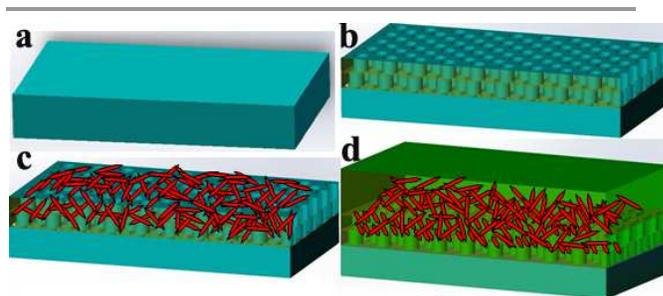
Sch. 1. (a) pure aluminium substrate; (b) anodic aluminium oxide after two-step anodic process; (c)  $\text{Co}_3\text{O}_4$  growth on AAO; (d)  $\text{Co}_3\text{O}_4$  growth AAO super slippery surface
