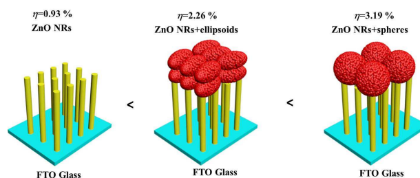
Scheme 1 Schematic illustration of the three kinds of photoanodes (ZnO NRs, ZnO NRs+ellipsoids, ZnO NRs+spheres).
