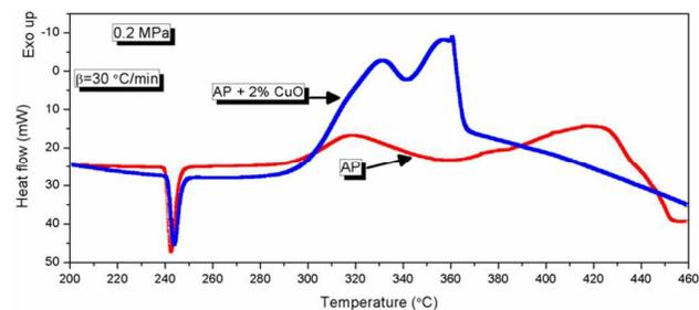
Figure 4. DSC heat flow curves obtained at 0.2 MPa for the samples AP and APC
