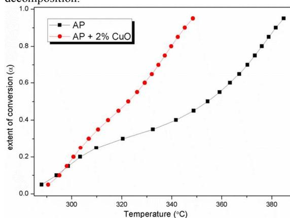
Figure 7.  $\alpha$  against T kinetic curves obtained for AP and APC obtained at  $\beta = 15$  °C/min
