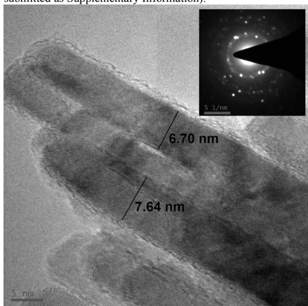
Figure 1. TEM image of CuO nanorods with electron diffraction pattern as inset
