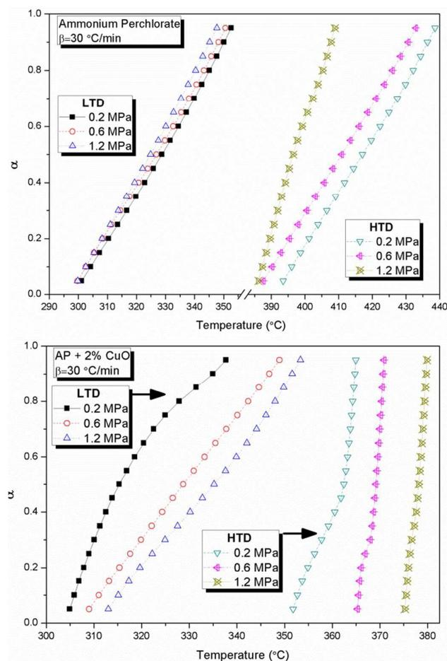
Figure 9.  $\alpha$  against  $T$  kinetic curves corresponding to LTD and HTD for the samples AP and APC under different pressure
