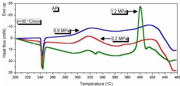
Figure 5. DSC heat flow curves obtained for AP at 0.2, 0.6 and 1.2 MPa
