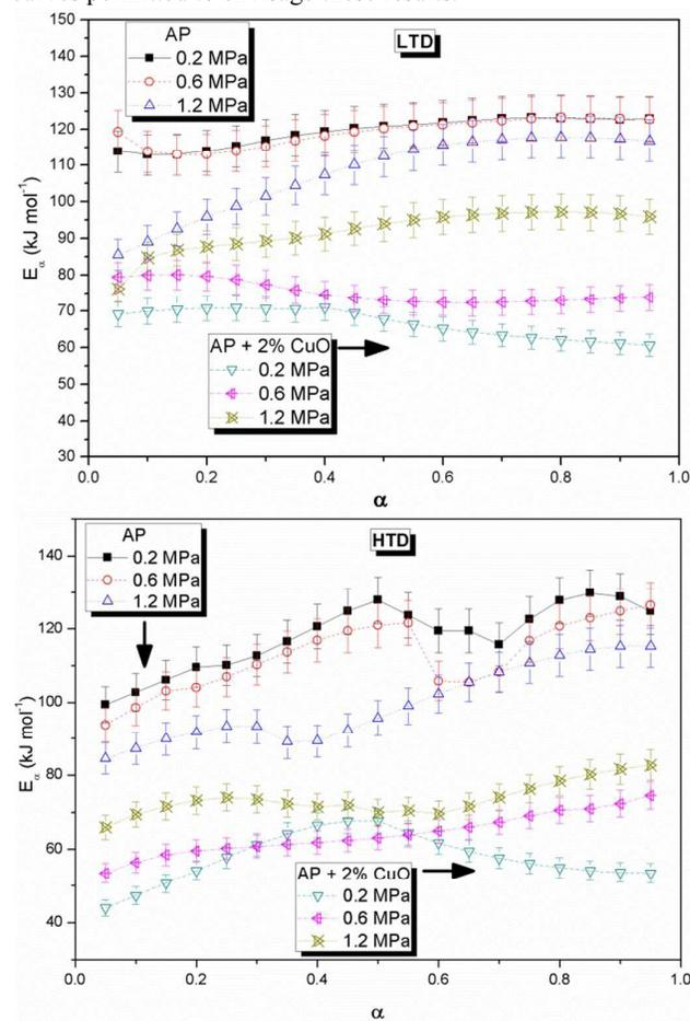
Figure 10. Variation of  $E_a$  with respect to reaction progress for LTD and HTD of AP and APC under different pressures
