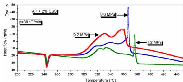
Figure 6. DSC heat flow curves obtained for APC at 0.2, 0.6 and 1.2 MPa
