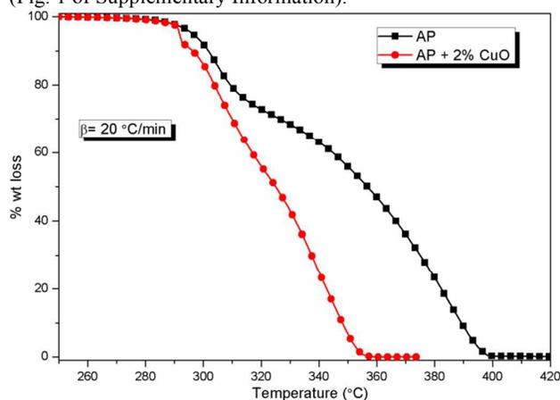
Figure 3. Nonisothermal thermogravimetric analysis curves for AP and APC samples
