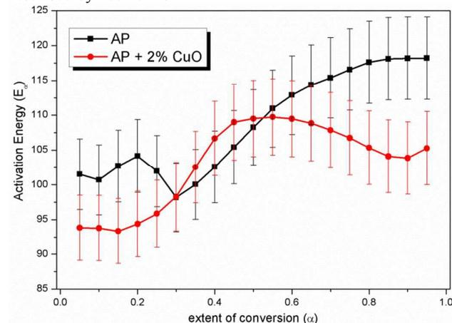
Figure 8. Variation of  $E_a$  with respect to reaction progress for AP and AP with nanocatalyst
